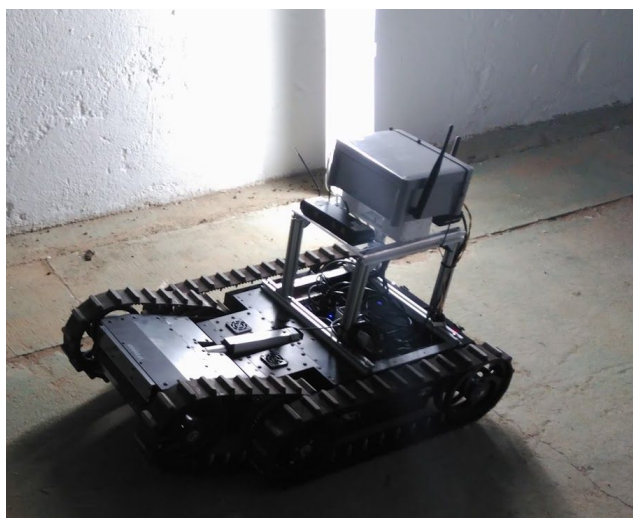
Figure 1.1. Experiments at UPO's premises with IDM's RAPOSA ® NG remote inspection platform.
