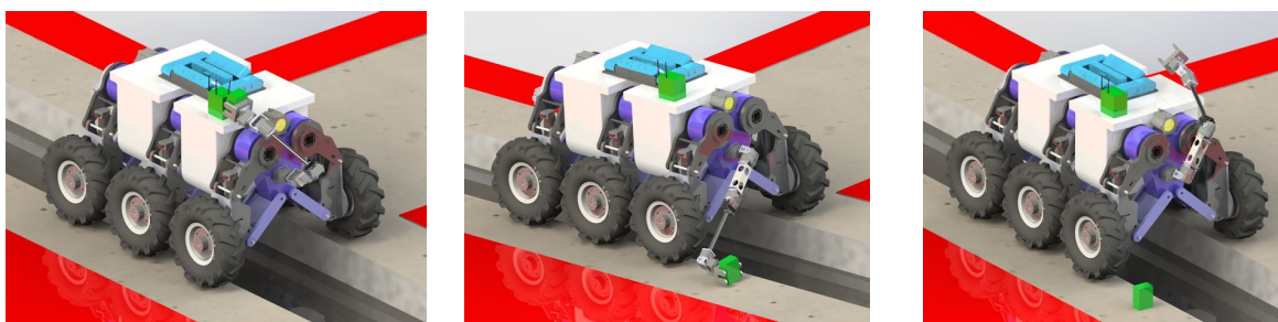
Figure 3.1. SIAR Robot deploying one wifi communication repeater
