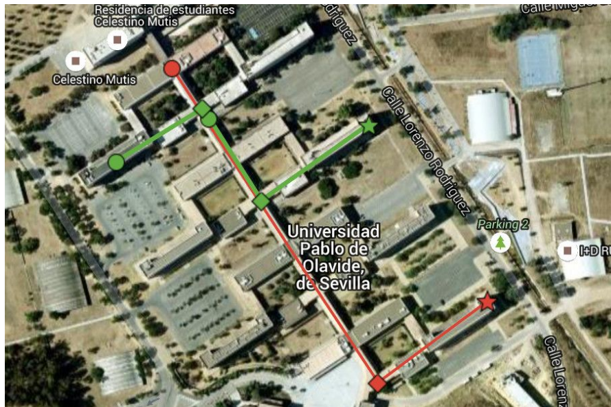
Figure 3.2. Location of the communication equipment and trajectories of the robot in the experiments at the UPO basement. Red: experiment with one repeater; the first leg is 330 m long, while the second is 120 m. Green: experiment with two repeaters; each leg is approximately 100 m long. The circles represent the position of the ground station.
