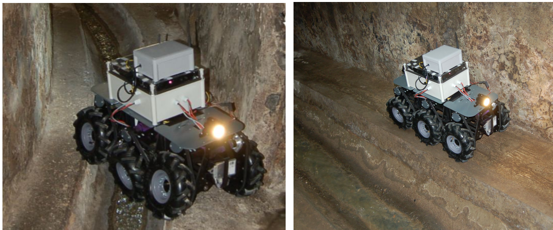
Figure 2.12. SIAR first prototype sewer testing.
