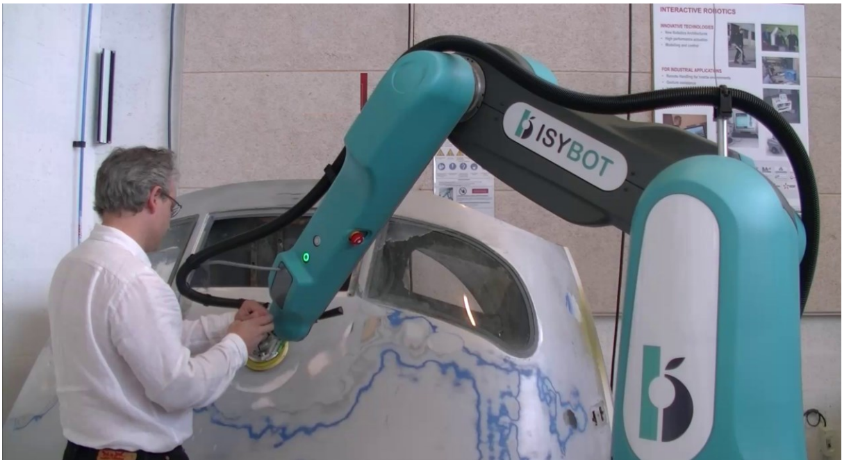
Figure 12: SYB3 product from iSYBOT polishing simulated product
