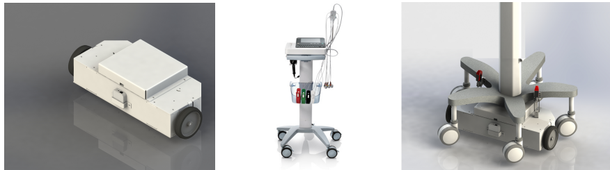
Fig. 11.4: From left to right: the ASSESSTORNIC mobile platform, a typical medical cart used in hospitals and the ASSESSTRONIC mobile platform mounted on a medical cart.
