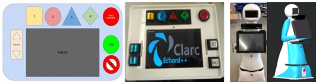
Figure 4 Interface re-designed (left), robot Chassis re-designed (right)
