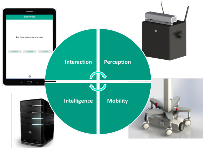
Fig. 11.1: The 4 modules composing the ASSESSTRONIC platform: the tablet PC for interaction, the workstation for perception of the patients' movements, the mobile platform for physical-based tests requiring big displacements and the server, which store all data and runs analysis algorithms.
