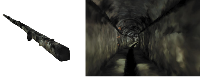
Fig. 12.12: 3D reconstruction samples of the sewer via current RGBD sensors and RTABMAP. Left: outside view. Right: inside view.
