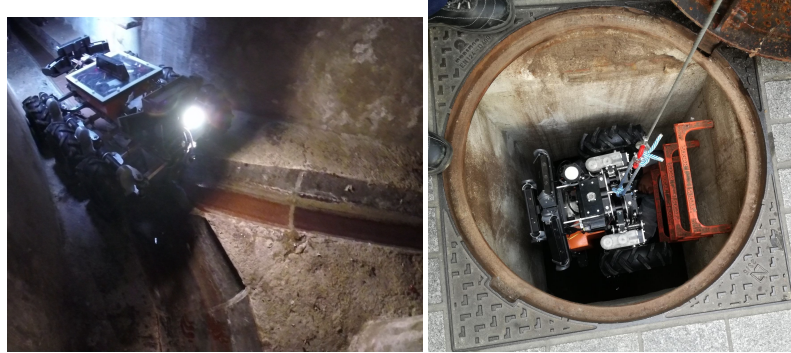
Fig. 13.1: Left: the SIAR platform in the sewer. Right: the robot being introduced in the manhole.
