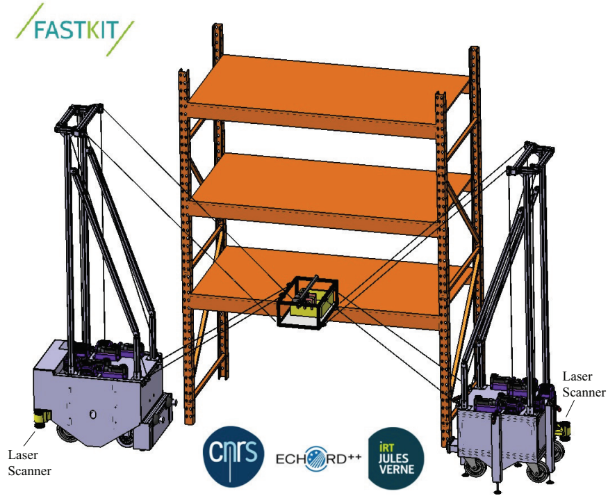
Fig. 8.1: FASTKIT concept: A cable-driven parallel robot mounted on two mobile platforms
