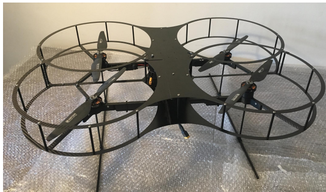
Fig. 12.2: ARSI quadrotor design with overlapping propellers
