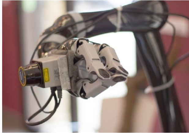
Fig. 5.11: 2D laser attached to the end tool of the arm.
