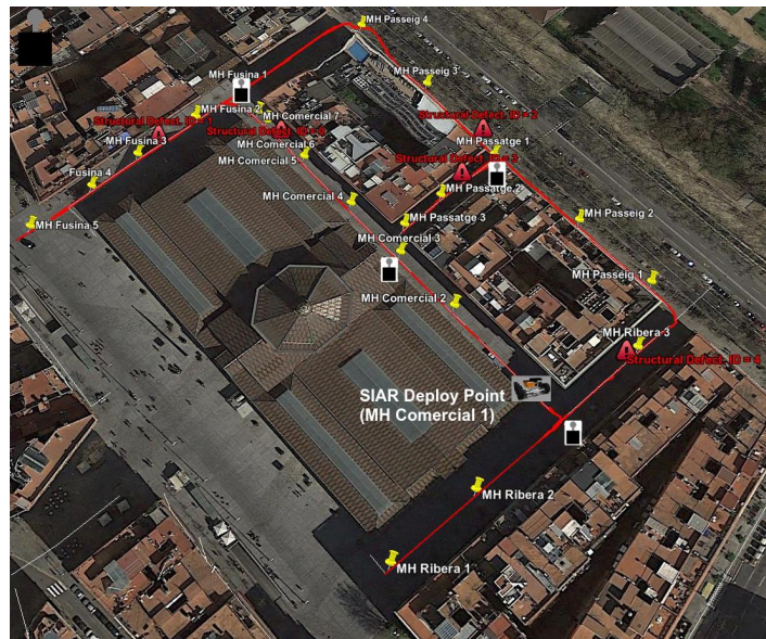
Fig. 13.11: Experimental setup of the presented experiments. Planned trajectory of the platform (red line) and visited manholes (marked with yellow stickers). Disposition of the repeaters with manhole deployment, depicted as black boxes with gray grippers. Reported defects found during the inspection marked in red exclamation signs. Finally, we deployed the robot over the manhole marked with a picture of the platform.
