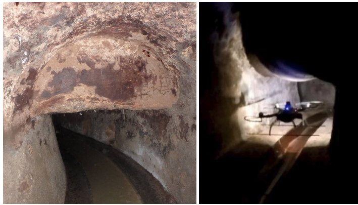
Fig. 12.10: ARSI MAV avoiding a service pipe crossing a sewer tunnel
