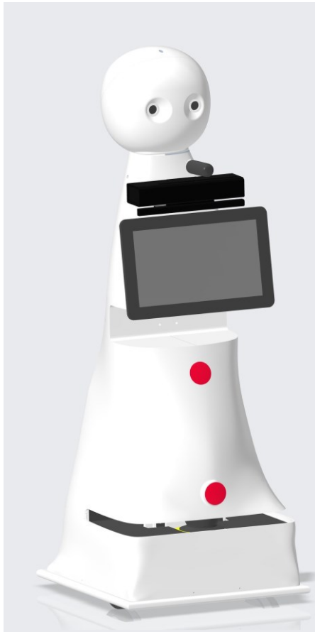
Figure 2.1 3D-Drawing and current realization of the CLARC robot prototype.
