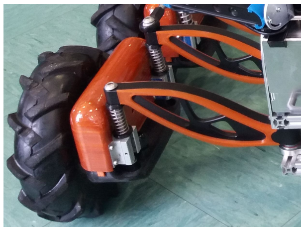
Figure 2.6 - New wheel and arms connection.
