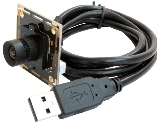
Figure 5.3: New camera that will be installed in the arm on top the robot.
