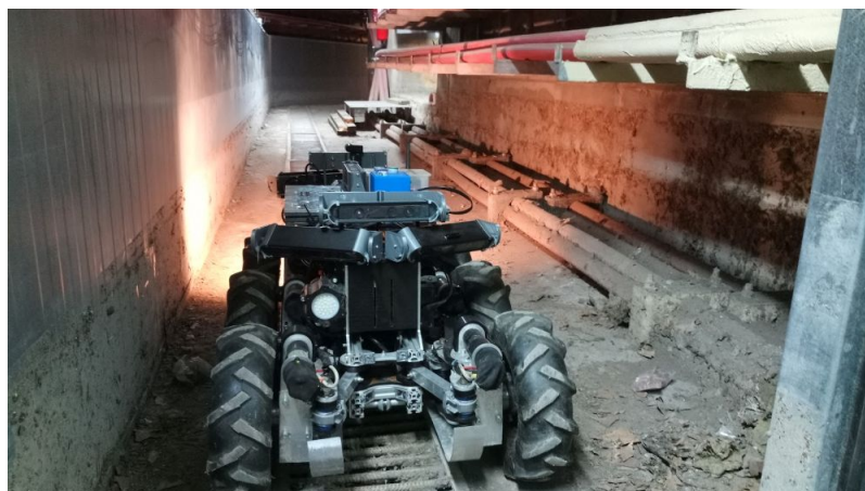
Figure 2.7. SIAR in an inspection mission in an underground energy distribution gallery.
