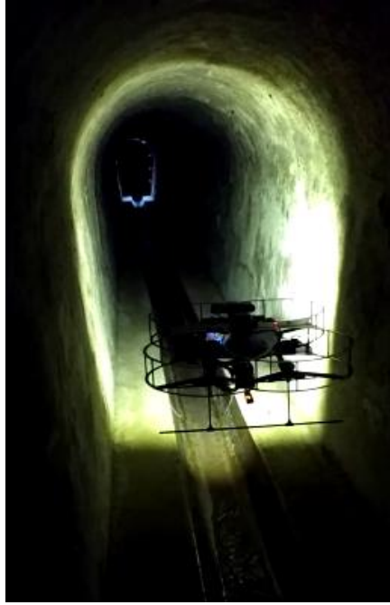
Figure 2: ARSI MAV executing a sewer inspection in Barcelona
