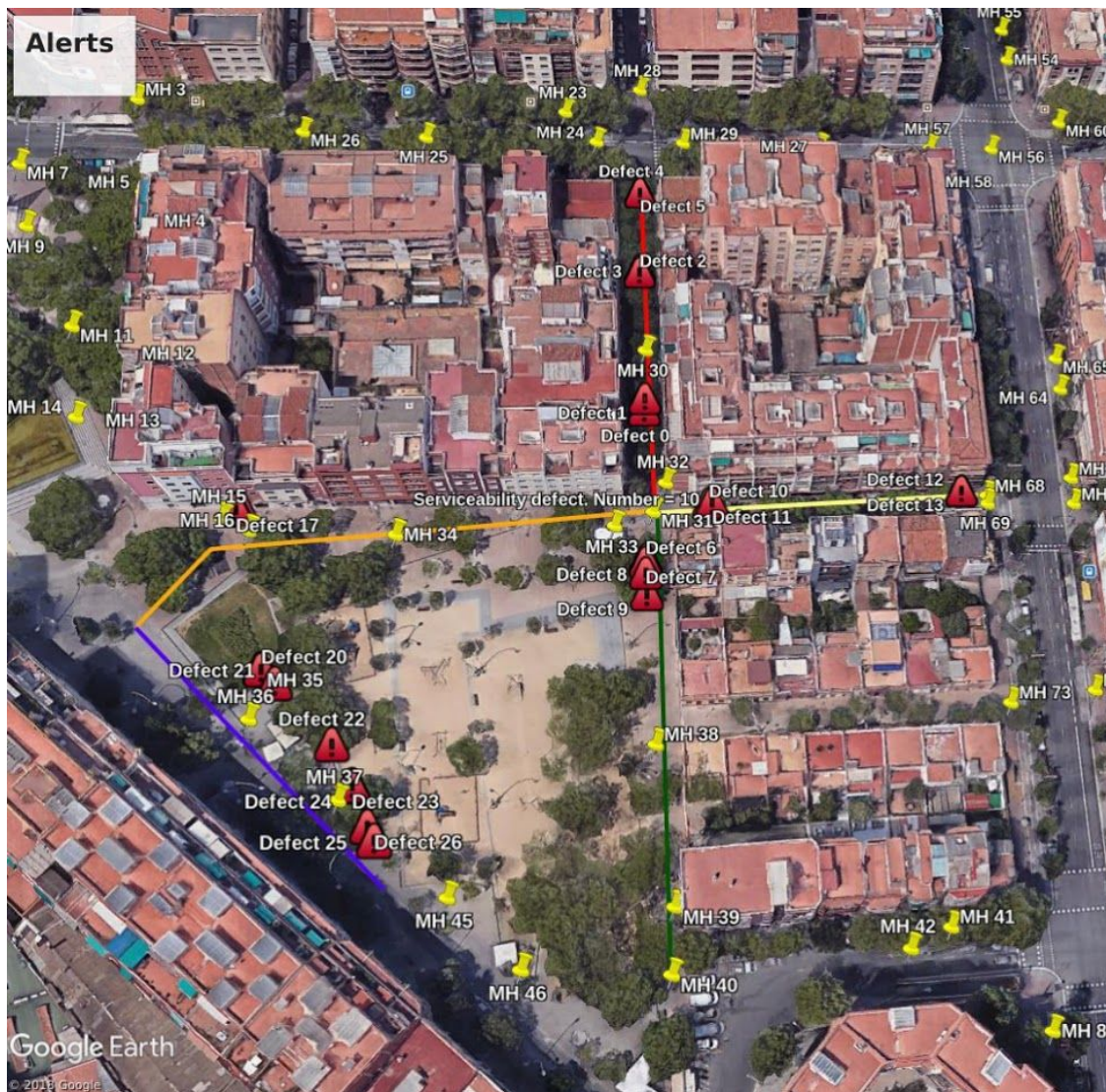
Figure 4.1: Automatically generated serviceability report for Virrei Amat area. The yellow spots show the location of the manholes. The red spots indicate the generated alerts.
