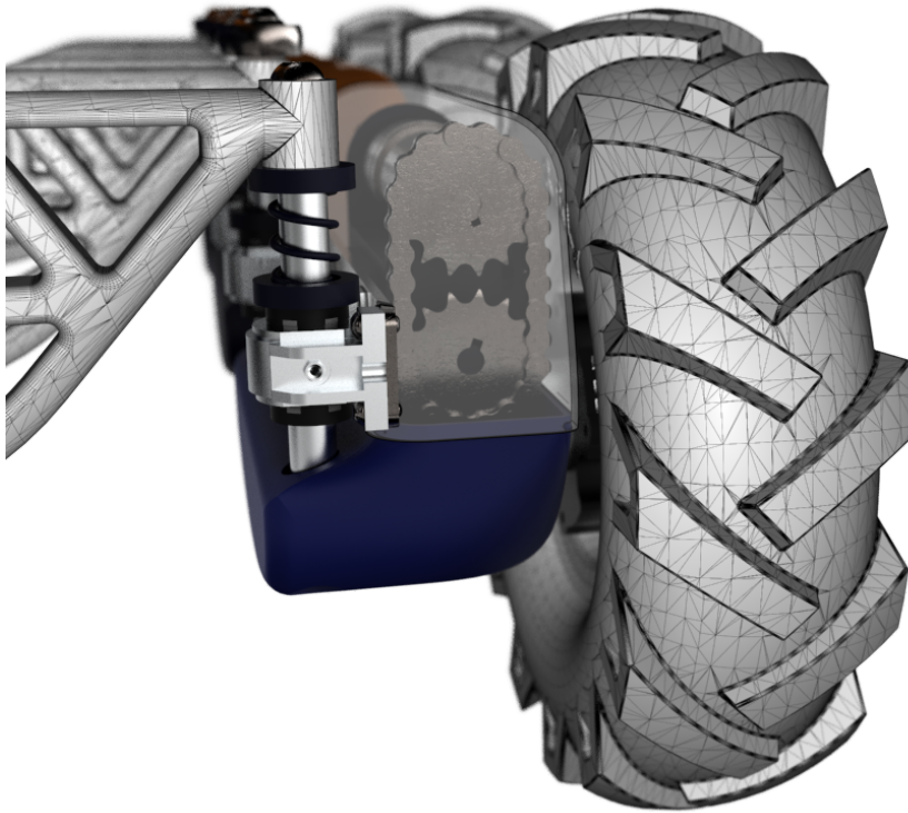
Figure 4.1 - Worm gear protection
