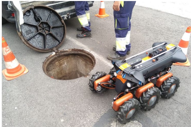
Figure 2.12 - SIAR with the protective shell
