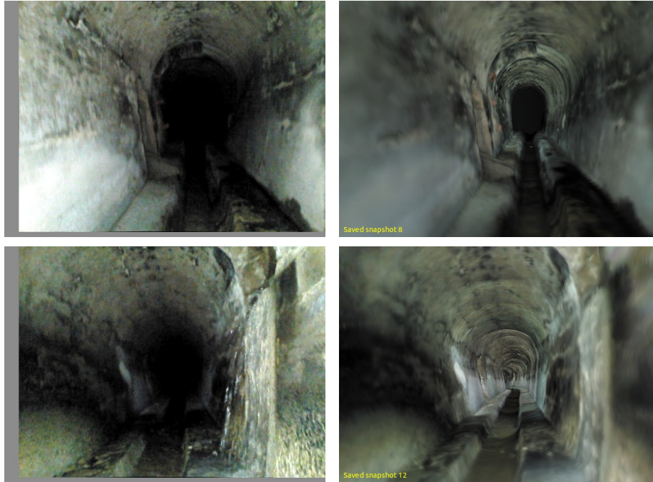
Figure 12: Comparison between images captured by the MAV (left) and the obtained reconstruction of the sewer model (right).
