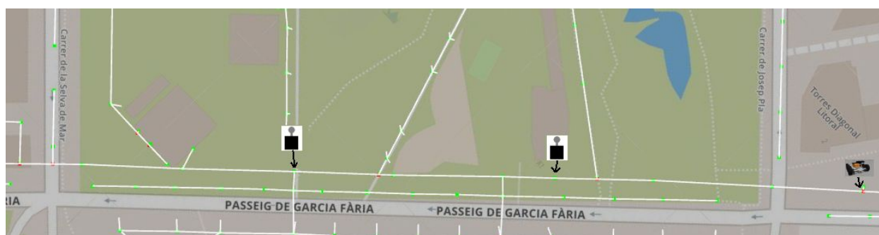
Figure 2.11: Inspection plan for Passeig de Garcia Fària area. The black boxes indicate the position of the repeaters and the robot points to the deployment manhole.
