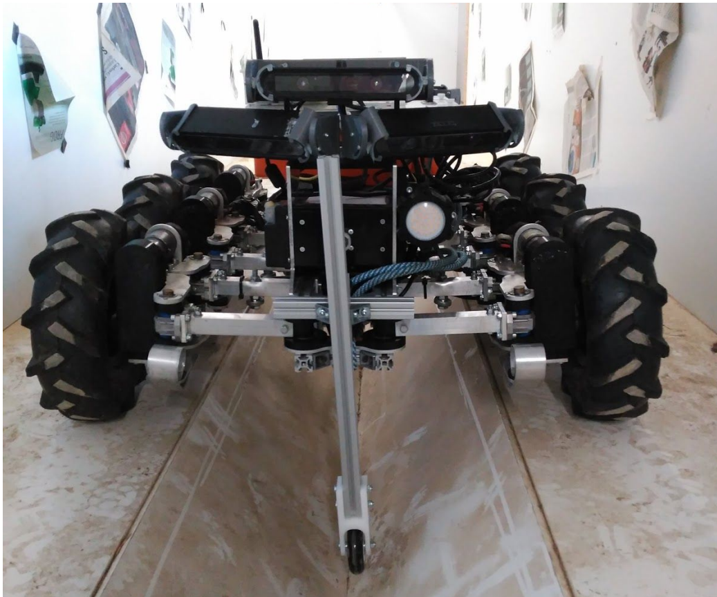
Figure 4.4 - Photo of SIAR v3 using the first solution in UPO's sewer mock-up
