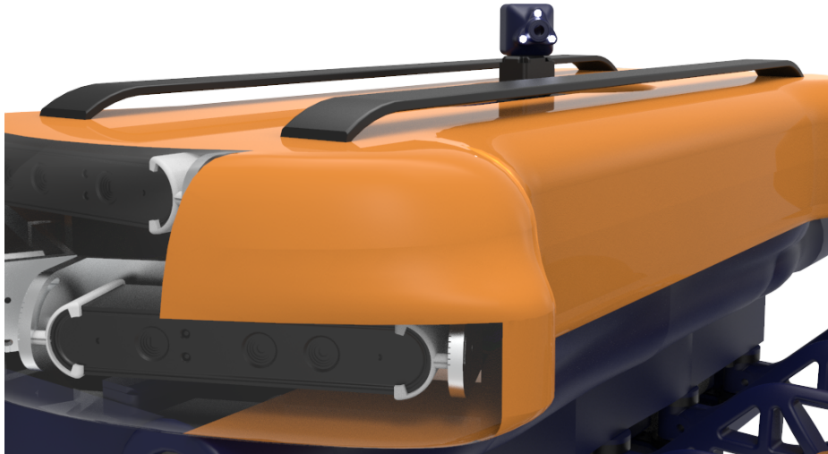
Figure 4.13 - Protective aluminium bars
