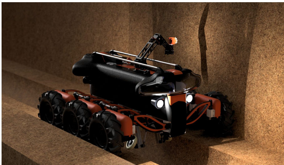
Figure 2.10: SIAR's inspection robotic arm with HD camera
