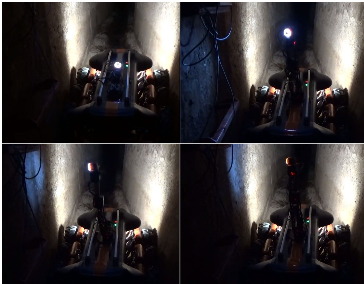
Figure 2.4 - Using the inspection camera arm
