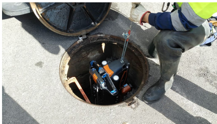
Figure 2.13 - Siar robot descending to sewer using the aluminum bars to protect the components
