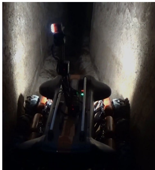
Figure 3.5. Detail of the inspection camera installed in the arm end.
