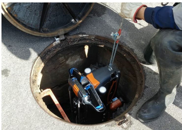
Figure 2.17 - Using the eye bolt to descend the SIAR robot
