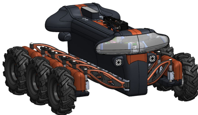
Figure 2.2. SIAR: the S ewer I nspection A utonomous R obot
