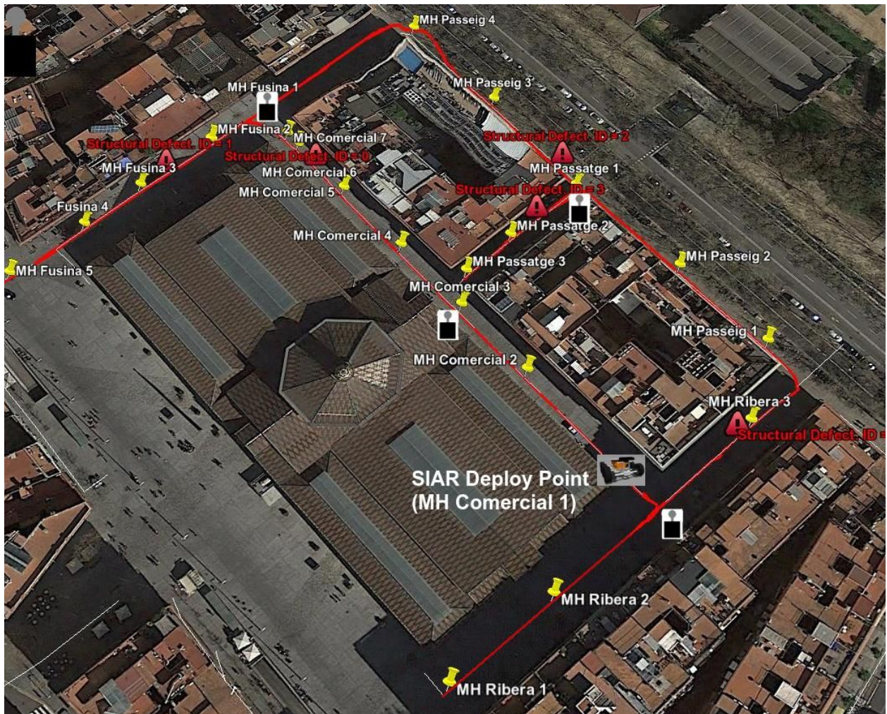
Figure 2.1: Trajectory of the platform (red line) and visited manholes (marked with yellow stickers) during the final demo of Phase II. Disposition of the repeaters with manhole deployment, depicted as black boxes with gray grippers. Reported defects found during the inspection marked in red exclamation signs.
