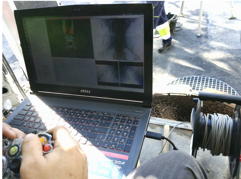
Figure 3.2: The robot is controlled from the Ground Station, which can run in a laptop, and shows visual and 3D information, including the view from the robot arm, as well as the automatically detected serviceability and structural defects alarms.
