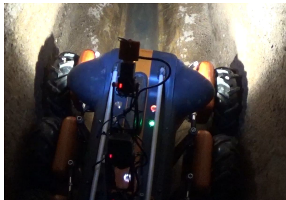
Figure 2.9: New SIAR 4.0 during navigation in the Av. Pearson area.
