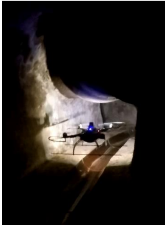
Figure 11: ARSI MAV flying at low altitude to avoid a service pipe in Mercado del Born
