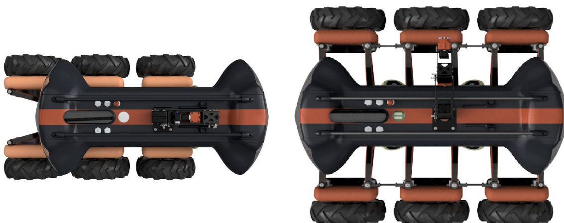
Figure 2.7: width adjustment system.
