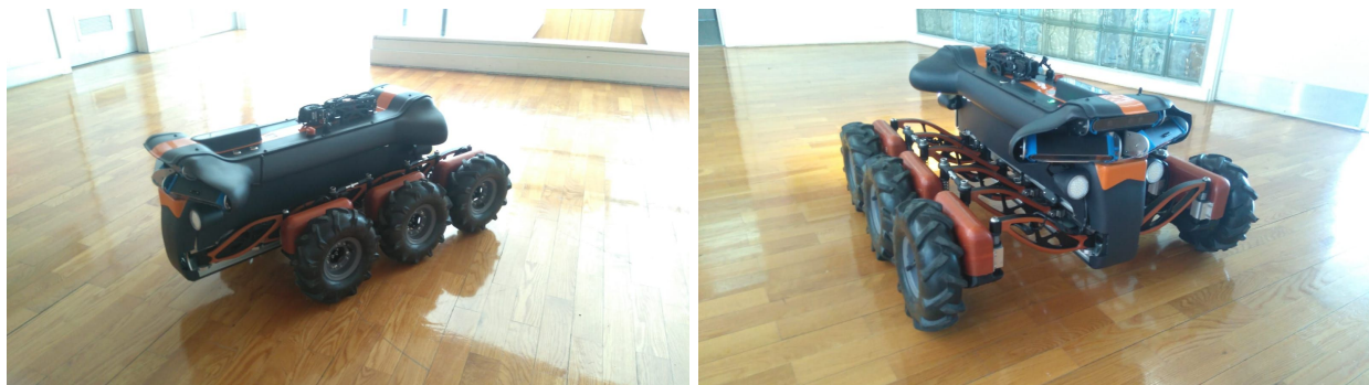
Figure 2.8: minimum width 520 mm (left); maximum width 850 mm (right).
