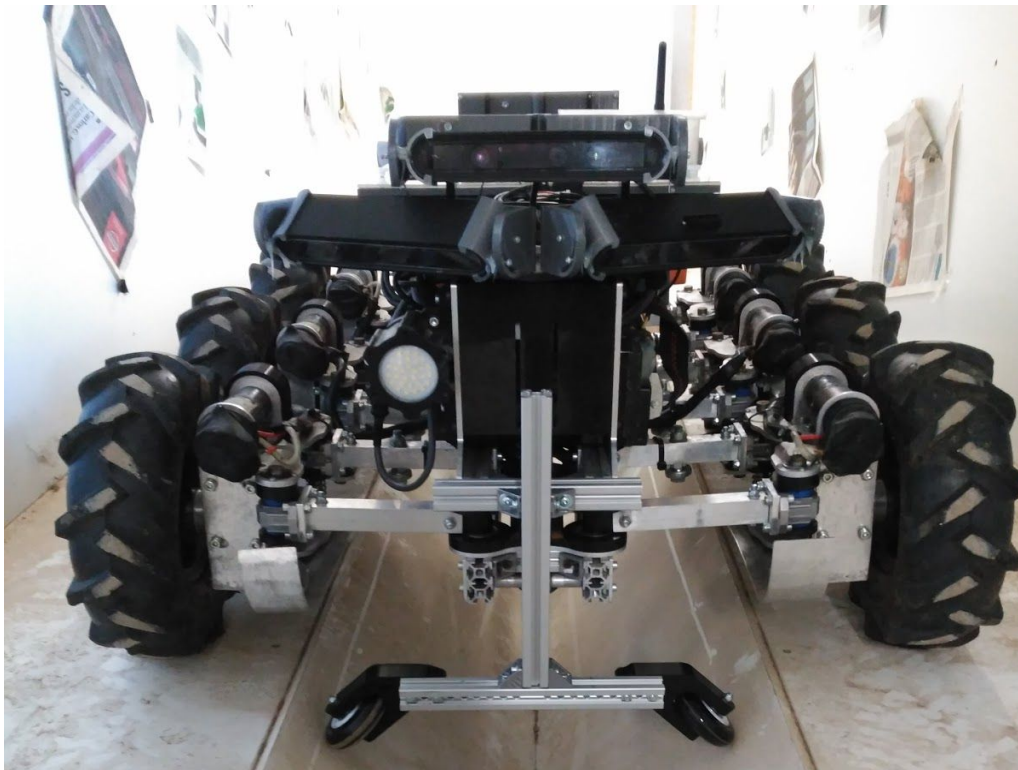
Figure 4.5 - Photo of SIAR v3 using the second solution in UPO's sewer mock-up
