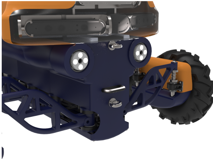
Figure 4.18 - Worst loading scenario - full robot weight on one wheel (600N)
