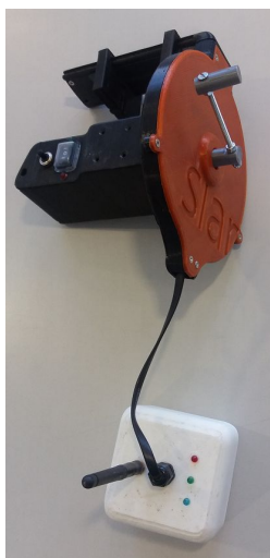
Figure 3.1 - Wireless repeater for manual deployment.
