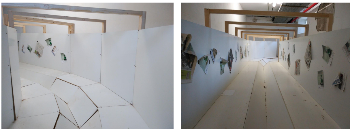
Figure 1: Photos of the 1-1 scale mock-up of the sewer used for navigation testing
