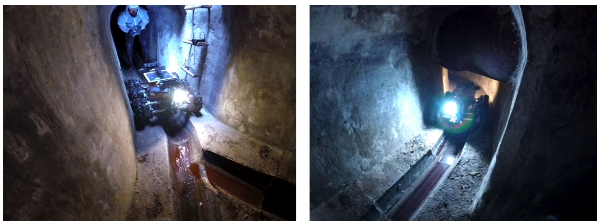
Figure 10: Frames of video in which SIAR robot is commanded to navigate over a cross-section in the sewer.
