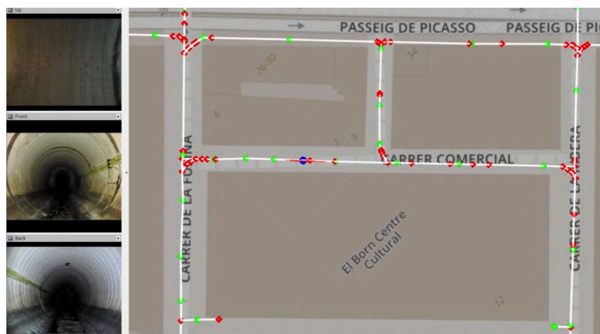
Figure 9: Frame of the video in which SIAR localization system works while navigating, crossing forks and pipes.
