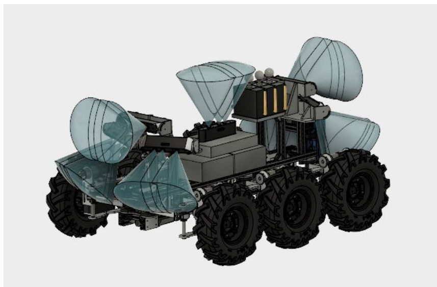
Figure 6.1: The robot carries 7 RGBD cameras. One on the top, and 3 cameras on the front and on the rear of the robot
