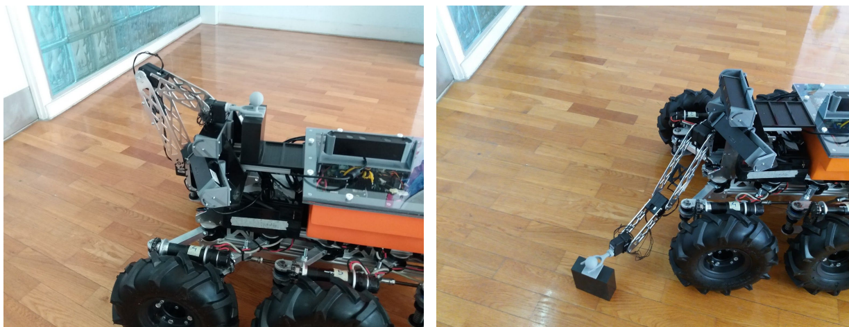
Figure 3.1: Left: Taking the wireless repeater from the robot top. Right: Deployment of the wireless repeater on the sewer floor.
