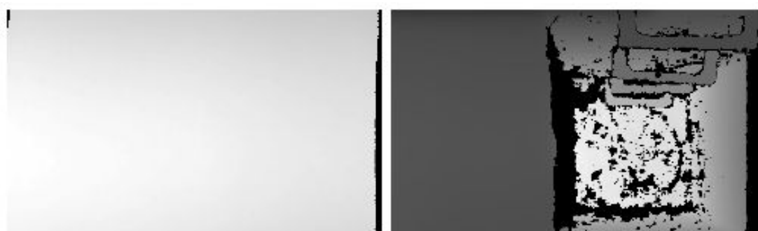
Figure 6.8. View of the sewer gallery from the depth camera pointing towards the ceiling. Left: regular gallery ceiling. Right: manhole.
