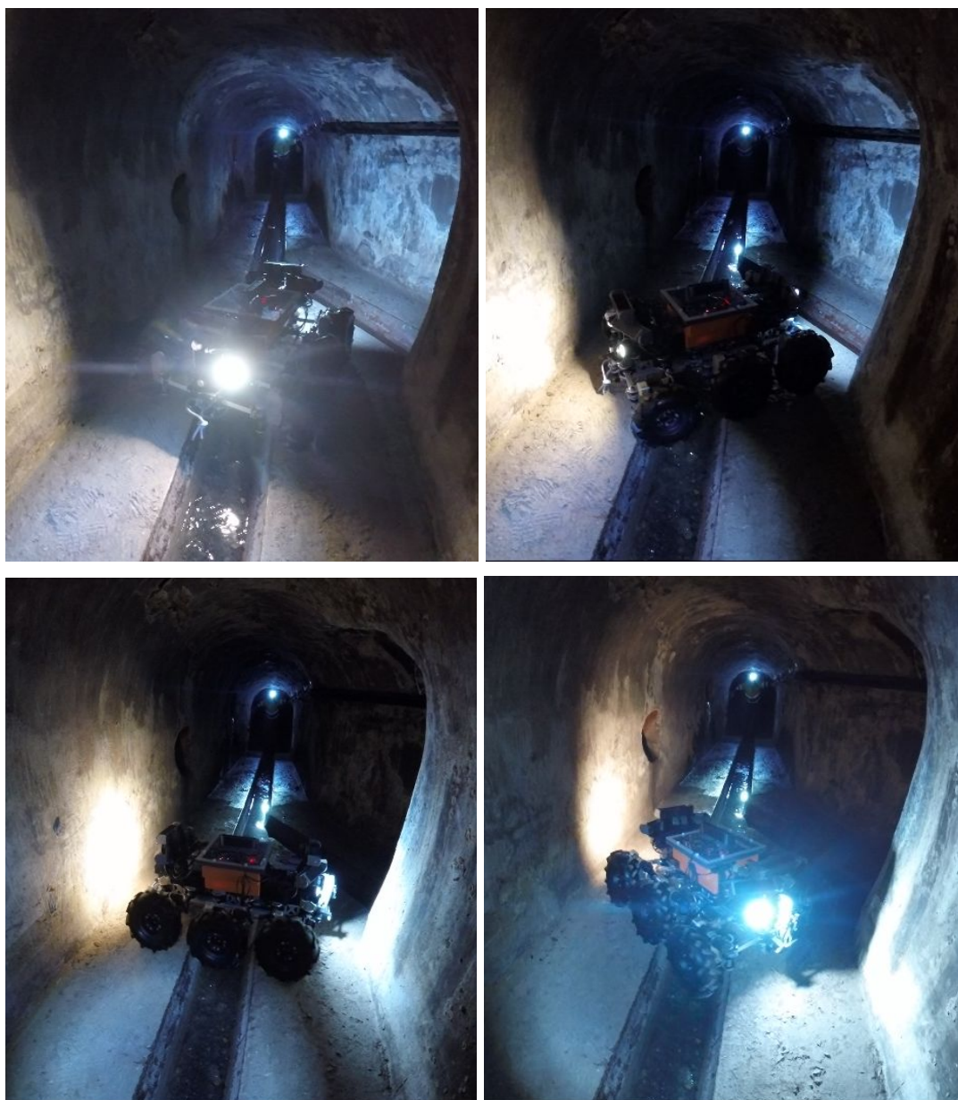
Figure 2.26. 180° rotation sequence over the gutter.
