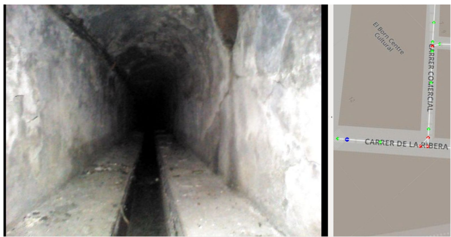
Figure 4.2. Main control window. Left, real-time images gathered from the front camera. Right: the location of the robot (blue) and the manholes (green) and forks (red).
