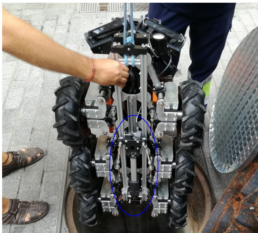
Figure 7.4 - Linear motor and its potentiometer and the bottom of the robot.
