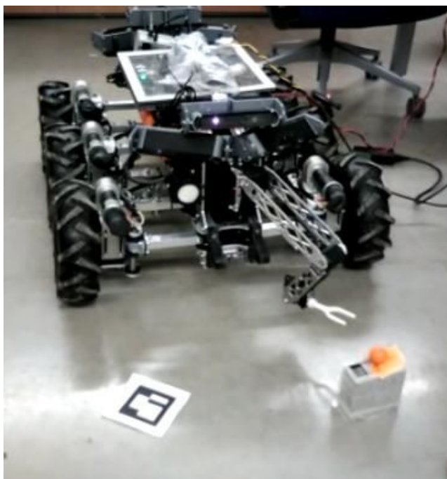
Figure 3.3. The robot is picking up a repeater from the floor
