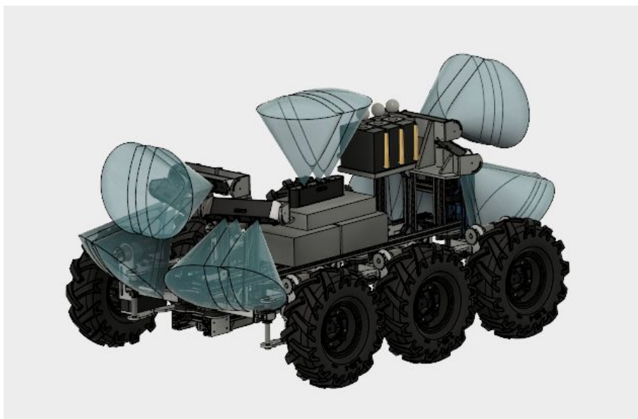
Figure 2.9. Proposed disposition of the cameras that compose the sensing system.
