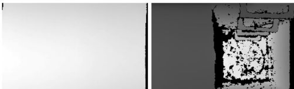
Figure 4.13. View of the sewer gallery from the depth camera pointing towards the ceiling. (Left) Regular gallery ceiling. (Right) Manhole.
