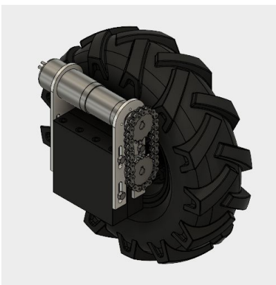
Figure 2.4. Implemented traction system.
