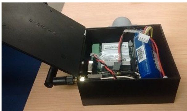
Figure 3.1. Components installed inside the wireless repeater.
