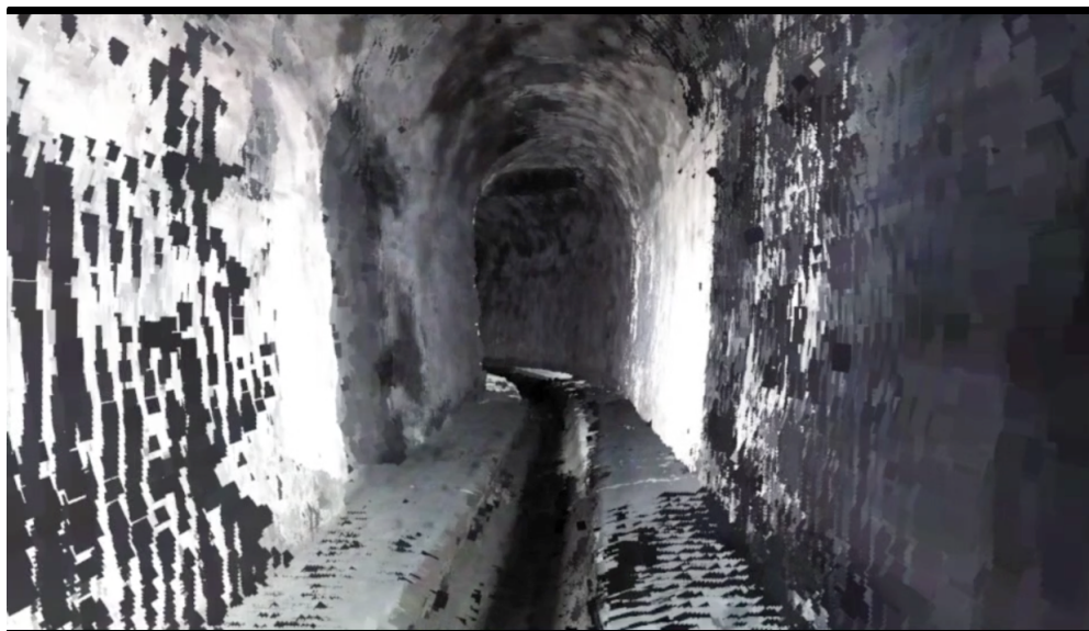
Figure 4.12. A section of the 3D reconstruction of the sewer
