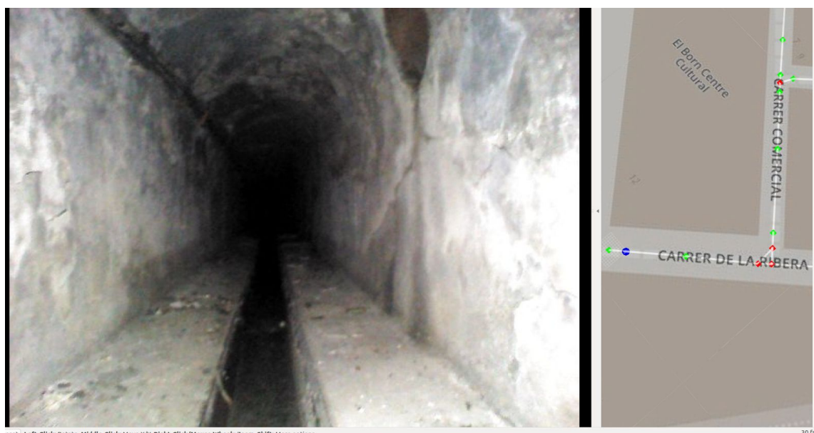
Figure 2.8. Main control window. On the left, real-time images gathered from the front camera. On the right, the location of the robot (blue) and the manholes (green) and forks (red).
