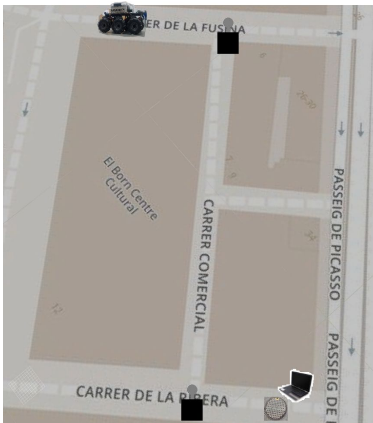
Figure 2.4. Disposal of the robot, base station (laptop) and repeaters (black boxes with grippers) in the furthest location reached in the experiment of the 23th of May, 2017.
