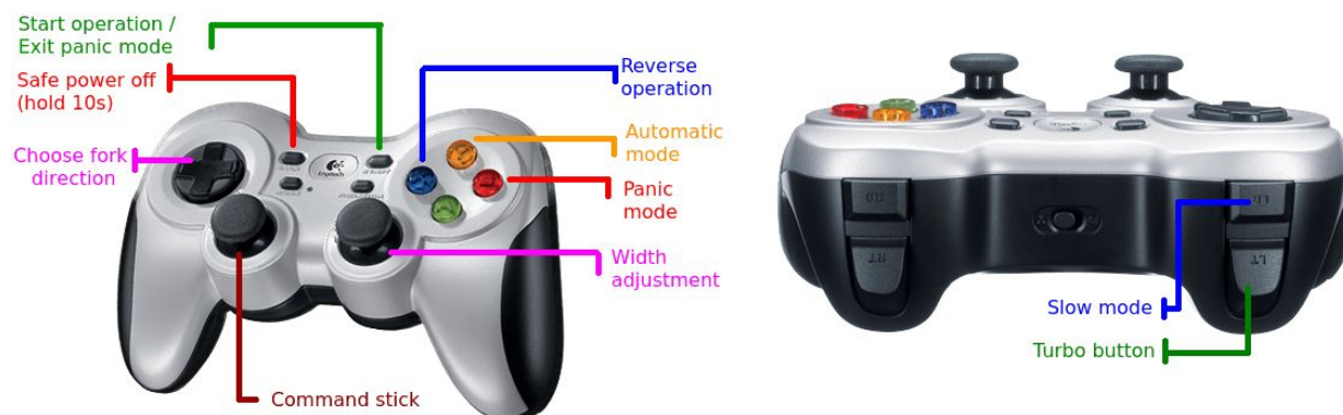
Figure 2.7. Controller used in the experiments and available commands.
