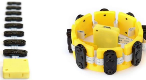
Figure 4: Example configurations of the TeraRanger Multiflex
