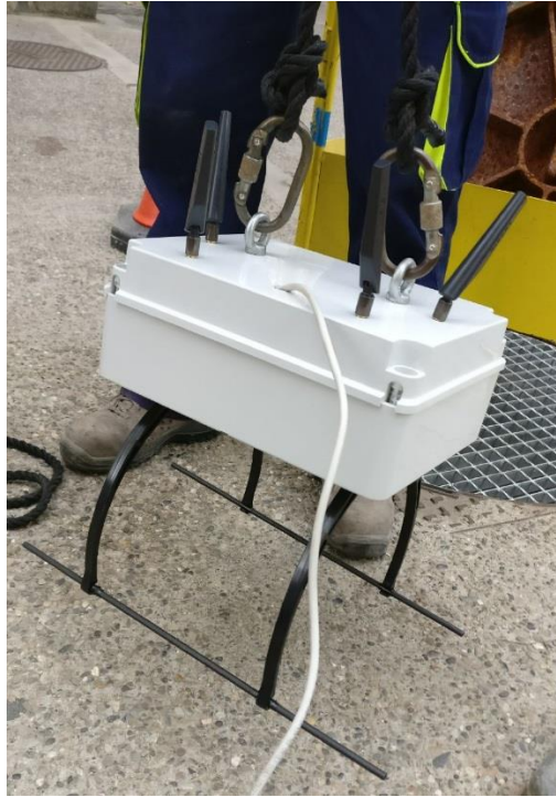
Figure 20: Rugged and watertight case for Wi-Fi router
