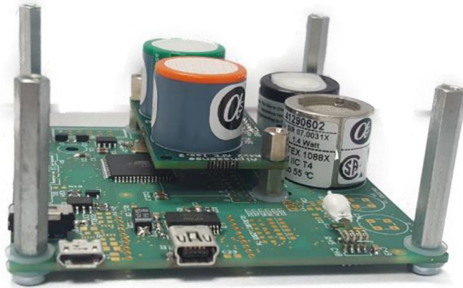
Figure 4: Gas detector developed in phase II
