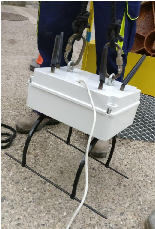
Figure 9: ARSI Wi-Fi router in its watertight case deployed in a sewer manhole
