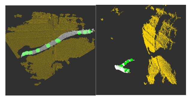
These cable center points have to be filtered to delete some possible false positives by using some constraints like the following: there have to be enough surface points in the initial point cloud around the found cable center points and the curvature of the segments has to be less than a maximum value.
