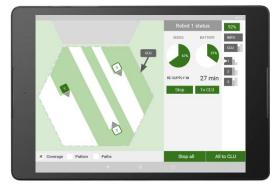
1) Detection and reporting that a robot is blocked. The specific type of error is visualized on the tablet. Robot is deactived and considered as obstacle.
