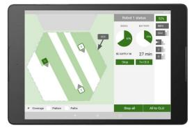
12) Also the status of each robot is monitored and visualized. The user can stop the robots individually or send them back to the CLU if needed.
