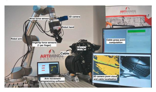
In the task the robot has to grasp a <u>cable</u> of a vehicle air conditioning system (HVAC) and clip it into a <u>hinge</u> at the HVAC.
