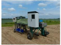
Middle bottom text (in the middle): GARotics harvester in the field with rain protection
