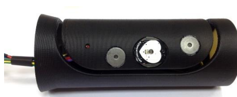
Figure 4 Cylindrically-shaped handle developed by UL integrates sensors for measuring skin conductance, photoplethysmography, skin temperature and grasping force
