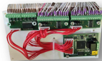
Figure 6: Developed controller board to measure sensor data and to communicate with PC.
