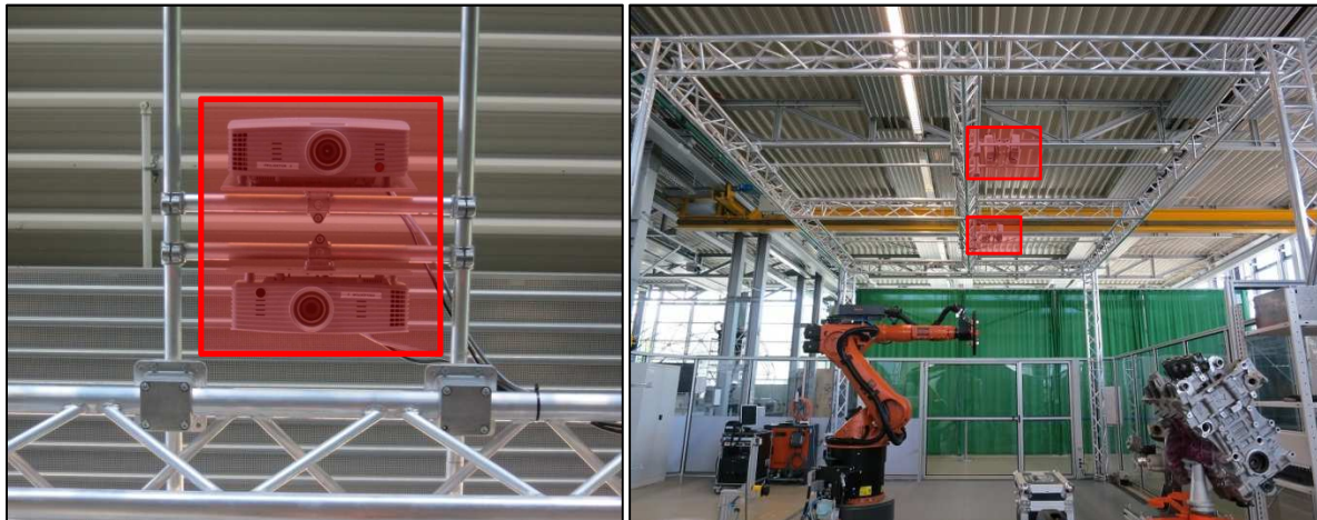
Figure 7: System carrier and mounted projectors in about 4 meters height.
