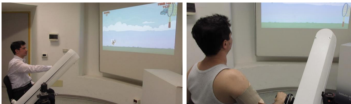
Figure 1 –LINarm++ mechatronic device interfaced to the virtual environment and with the user holding the cylindrical sensorized handle. In the right picture the rehabilitation task is supported by a wearable embedding a set of electrodes for functional electrical stimulation.
