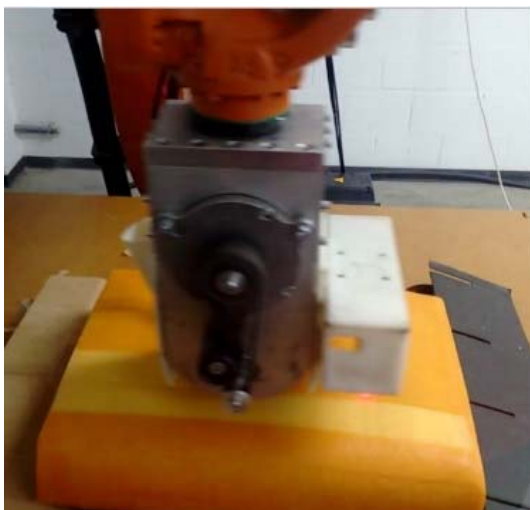
Figure 4: The robot motion on the cheese block while removing the coating.
