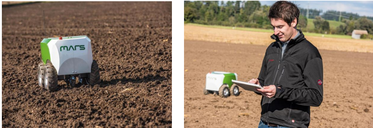
Figure 3 Mars Swarm Robot on the field, right: Thiemo Buchner from AGCO Corporation, controlling the Mars Swarm
