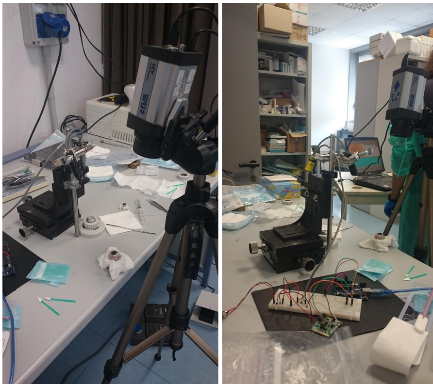
Figure 7. The test setup on the porcine eyes. It is possible to see the laser diode and the electronic controlling system, together with the IR thermal camera used to monitor the welding effects.
