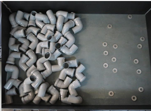
Figure 2 Randomly stored parts in a bin (left: angle tubes, right: washers)
