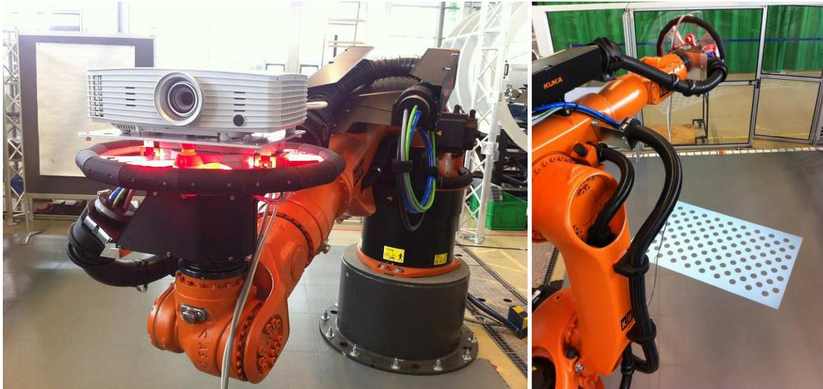
Figure 9: Robot equipped with projector for intrinsic projector calibration. The projector is positioned at arbitrary perspectives.
