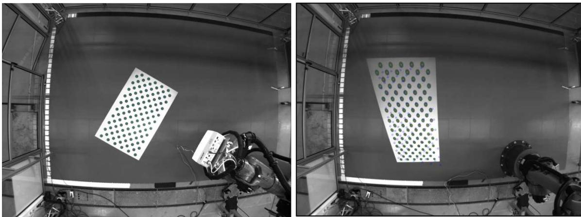
Figure 10: Projected calibration pattern from perspective of high-resolution camera. Circle detection for determining the intrinsic parameters of the projector.
