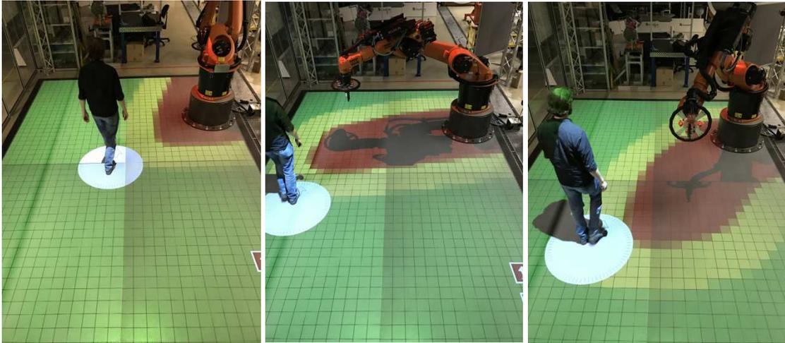
**Figure 24: Human is moving straight forward to the robot while the dimension of the safety zones is adapted dynamically on basis of the human's behaviour. Left: Robot is in initial position [1]. Middle: robot is in intermediate position [2]. Right: robot is in target position [2].**
