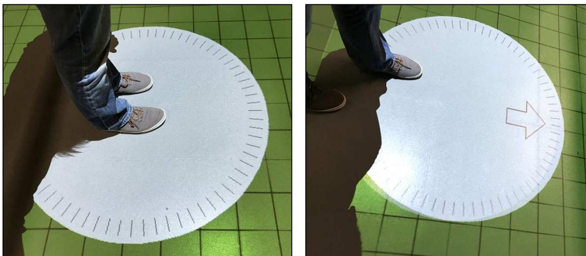
Figure 30: Visualization of detected human's position (left) and estimated movement direction (right).
