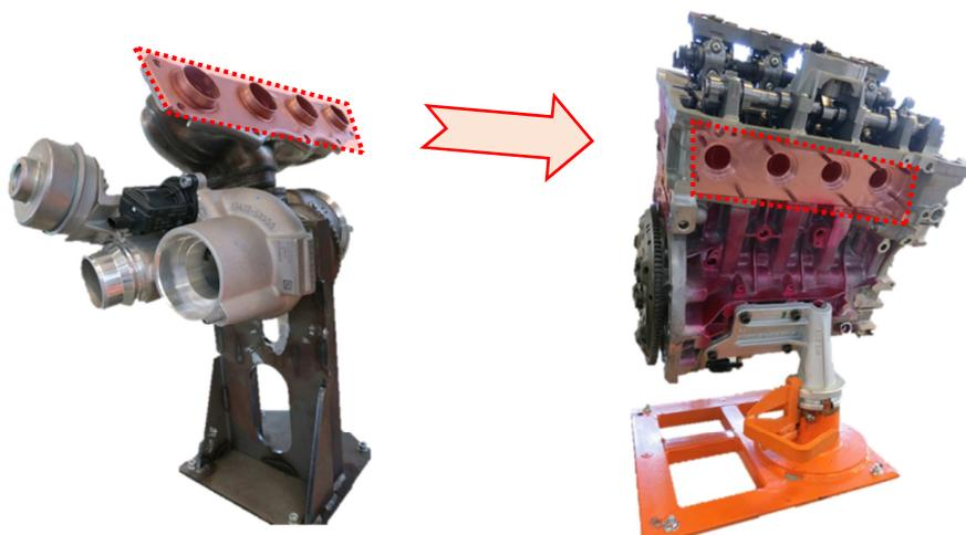
Figure 6: The scenario comprises the assembly of a turbocharger (left) and motor block (right).
