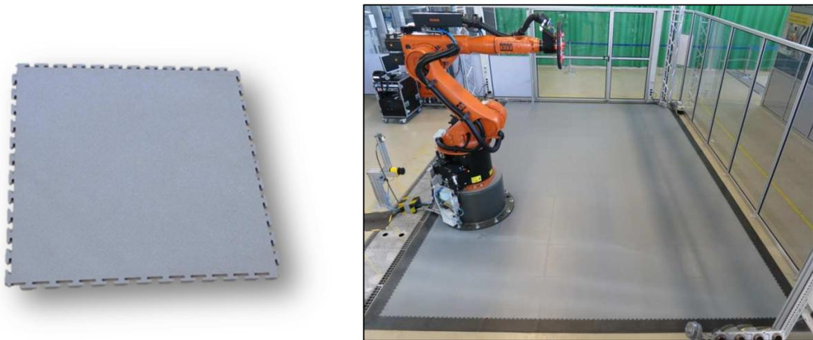
**Figure 3: Industrial grade mat (left) and resulting covering of the entire tactile floor (right).**
