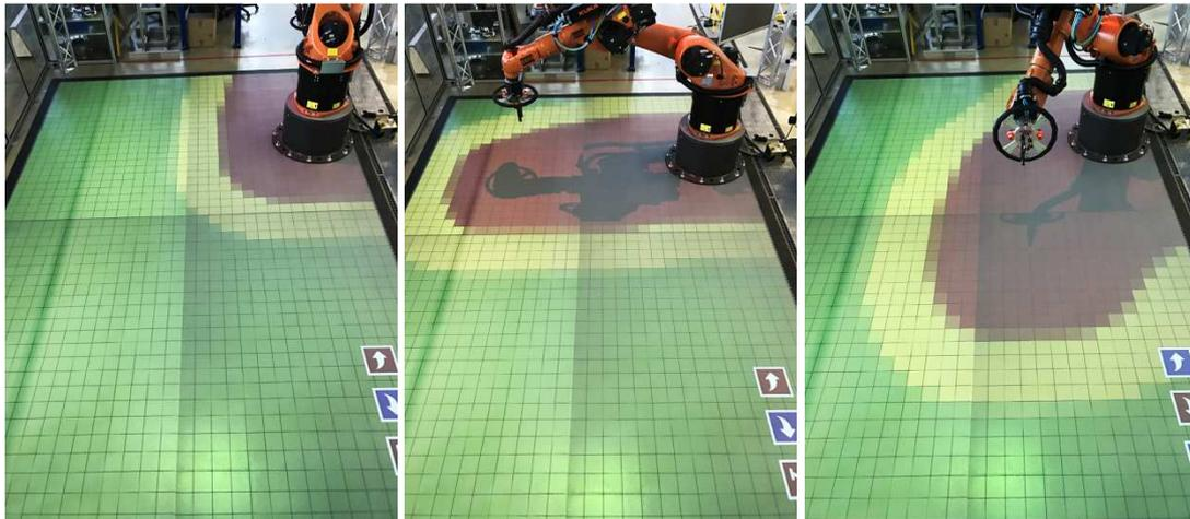
Figure 20: Dynamic safety zones on basis of current robot's joint angles and velocities at different robot positions. Amount of sensor cells: Left: 524; Middle: 924; Right: 967
