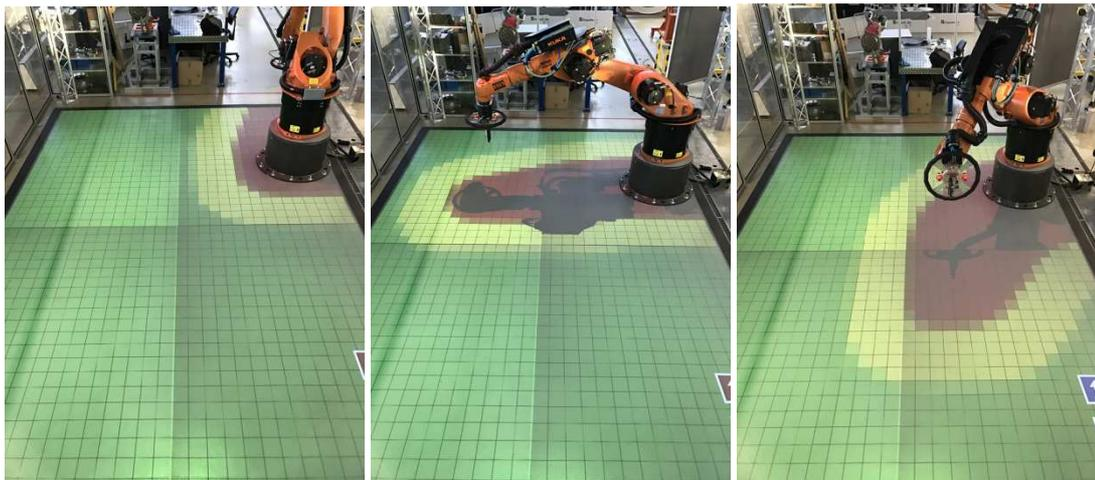
Figure 22: Dynamic safety zones on basis of current robot’s behaviour and current human’s behaviour. Amount of sensor cells: Left: 397; Middle: 739; Right: 723
