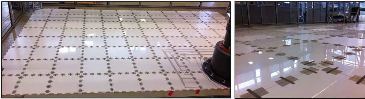
**Figure 2: Setup of the tactile floor that comprises 96 quadratic tiles with 1536 sensor cells altogether.**
