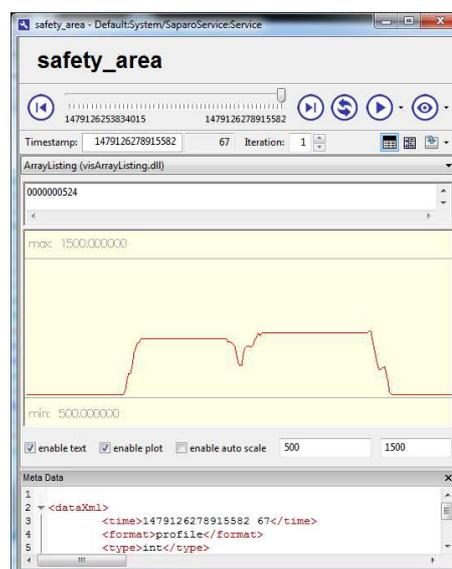
Figure 21: Safety approach 3: Amount of sensor cells that represent critical zone and warn zone while the robot moves from initial position [1] via intermediate position [2] to target position [3].
