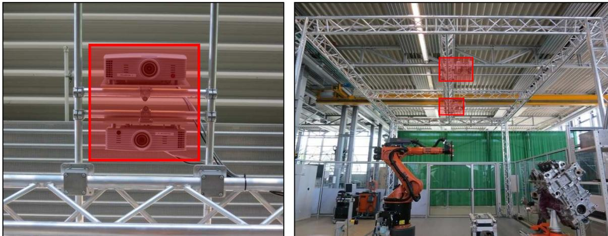
Figure 5: System carrier and mounted projectors in about 4 meters height above the human-robot workplace.
