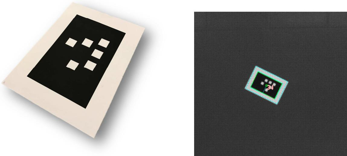
**Figure 14: Marker detection for measuring the position and velocity of the human.**
