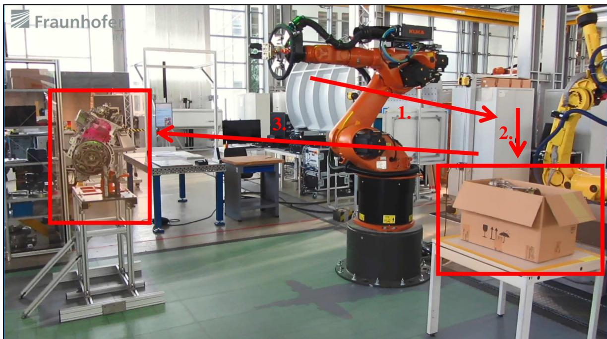
Figure 7: Single steps of the assembly process: Mounting a turbocharger to motor block.
