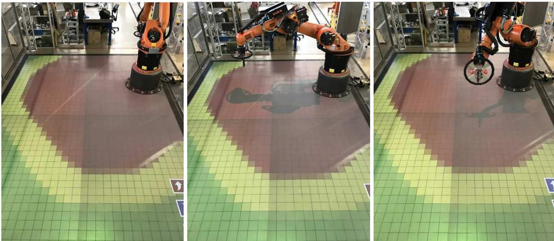
Figure 19: Movements of the robot monitored by semi-static established safety zones.
