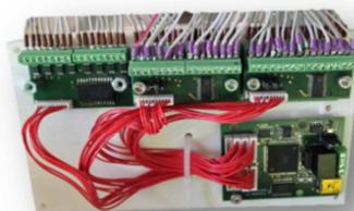
**Figure 4: Developed controller board for collecting sensor data and communicate with computing hardware by USB.**
