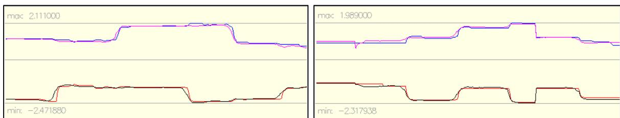
Figure 15: Comparison of human's position determined by tactile floor and tracking system.
