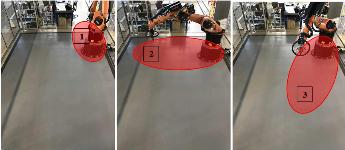
Figure 18: Pre-defined robot trajectory for evaluating the different safety approaches. Robot moves from initial position [1] via intermediate position [2] to the target position [3].
