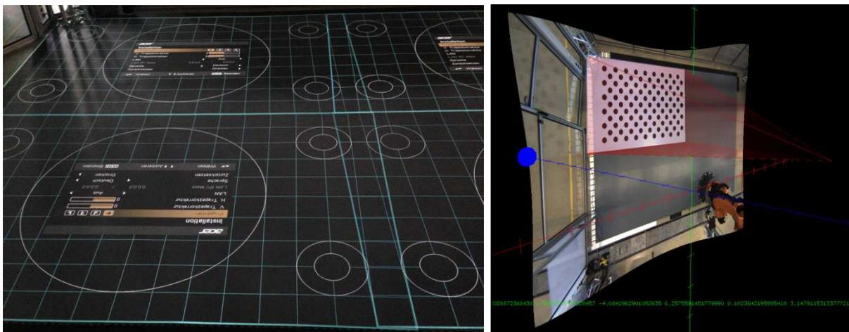
Figure 11: Extrinsic projector calibration. Left: Manual adjustment of the projectors. Right: Projection and detection of calibration pattern for optimizing the position by algorithms.
