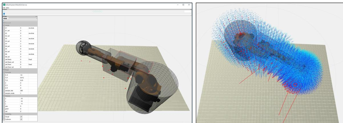
**Figure 17: Simulation environment used to develop and implement the single safety approaches that are based on the distance formula described in ISO TS 15066. Right: Resulting safety distances (blue) at robot movement by a joint (A1) velocity of 0.8 rad/s.**
