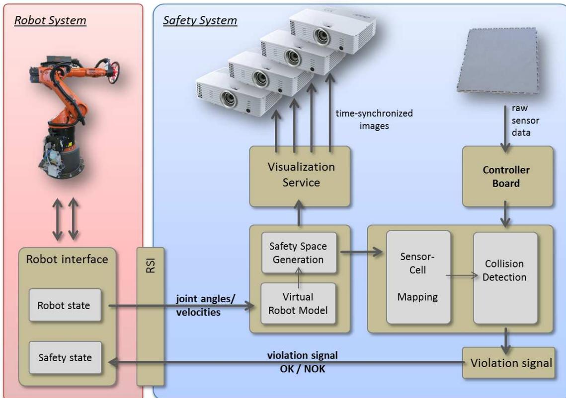
**Figure 8: Overall scheme of the safety concept representing the main communication interfaces of software and hardware components.**
