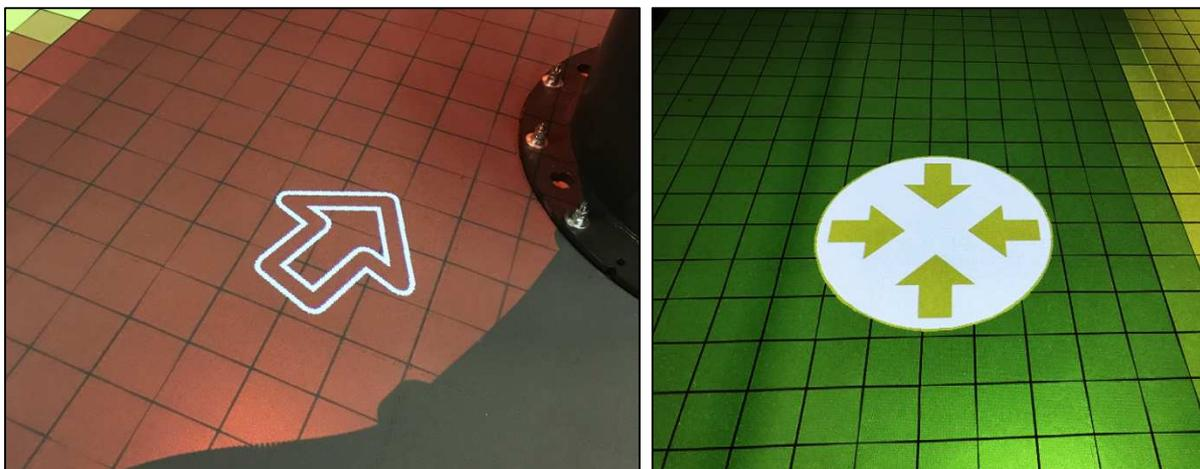
**Figure 27: Visualizing next robot's movement direction (left) and target position (right).**
