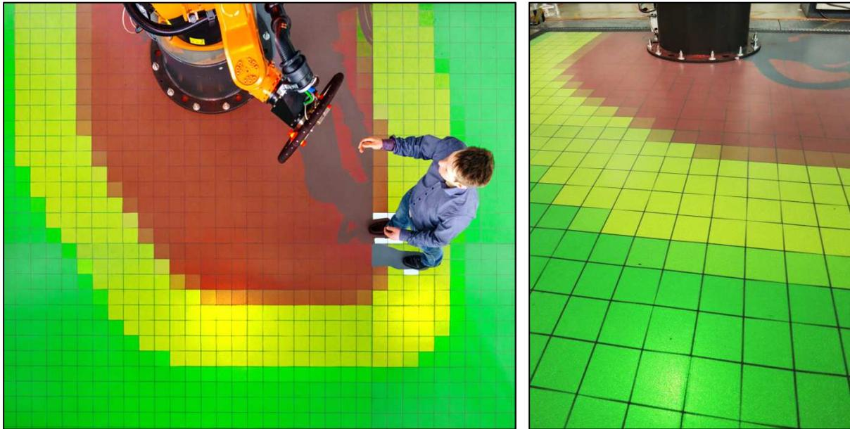
**Figure 26: Grid-based representation of the sensor cells of the tactile floor. Dynamic generated safety zones that consist of a critical zone (red area), warn zone (yellow area) and free zone (green area).**
