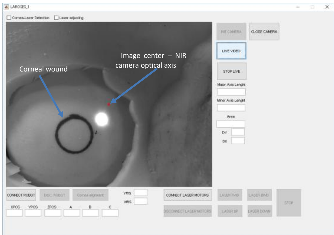
Fig. 1 – initial positioning of LA-ROSES laser system. The NIR camera centre is not aligned with the cornea center
