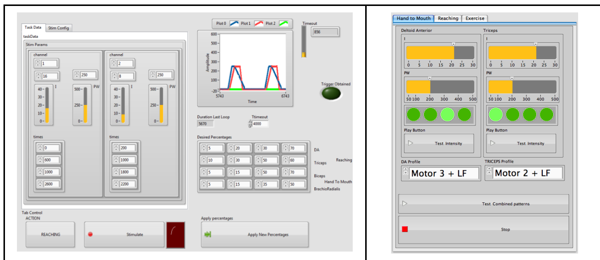
Figure 6: Left: a simple GUI that allows in “engineering mode” to quickly prototype and test different activation profiles. Right: a simplified GUI that allows choosing stimulation intensity, location of stimulation, and preset patterns, and then testing the overall pattern.
