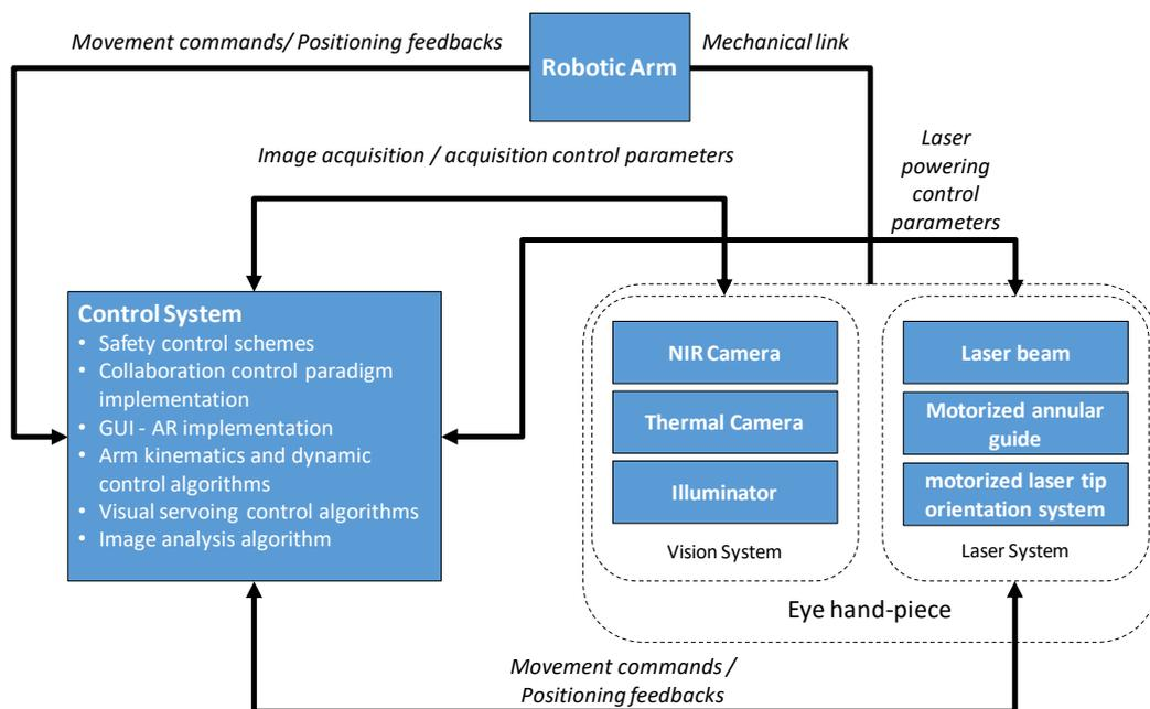
Fig. 1 - Overall system diagram of LA-ROSES functional subsystems
