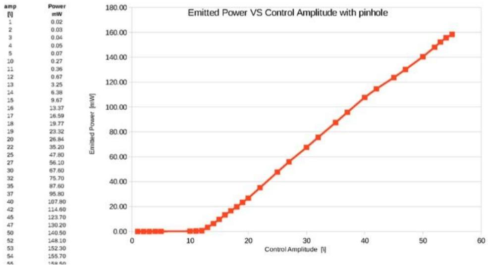
Fig. 11: Optical power vs control voltage and optical system for laser spot control.
