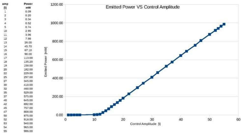
Fig. 10: Optical power vs control voltage.
