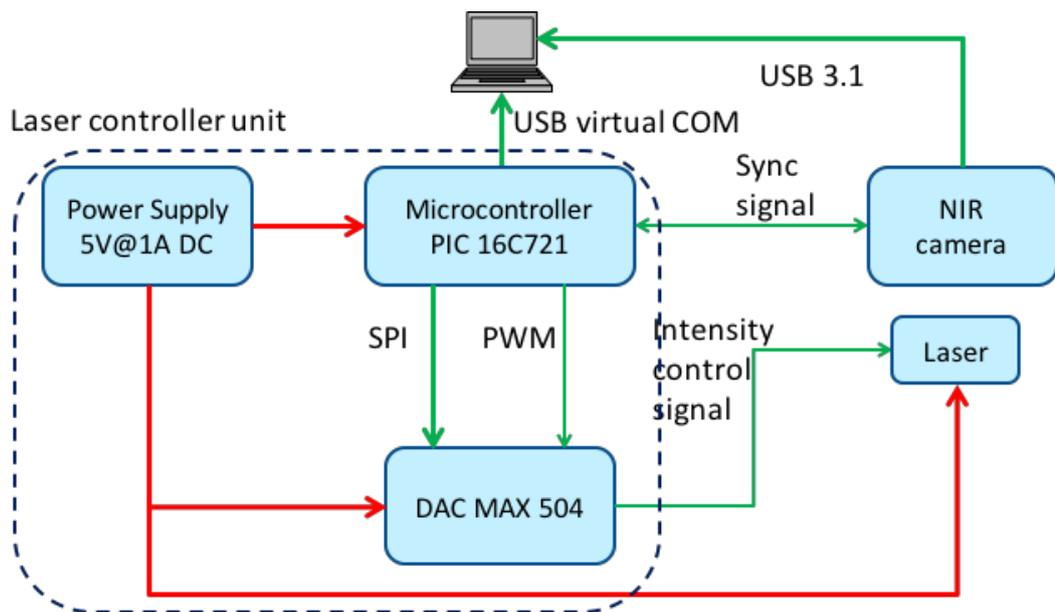
Fig. 4 – The laser controller unit (dotted blue line) and its connection
