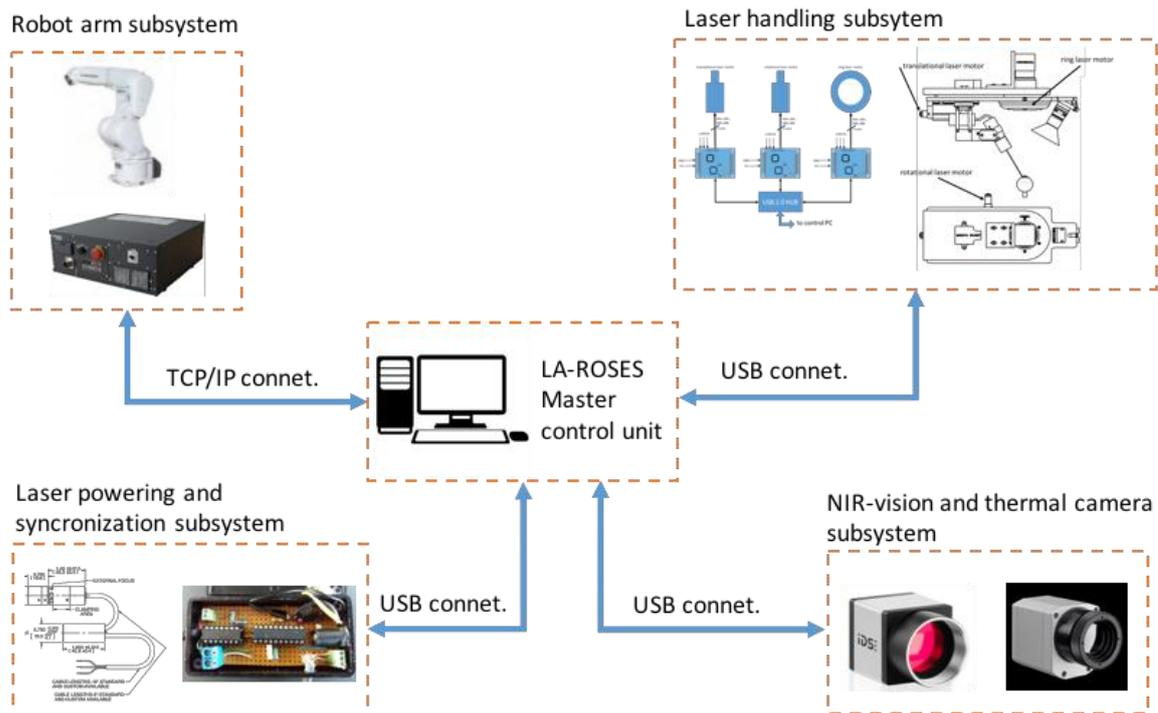
Fig. 2 - Overall system diagram of LA-ROSES subsystems. Arrows show the type of communication channel used to exchange commands and data between the LA-ROSES master control unit and each subsystem
