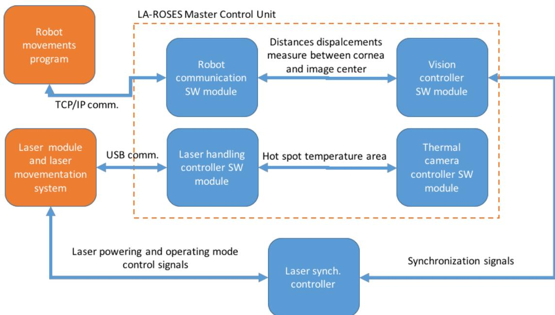
Fig. 8 – LA-ROSES SW controllers diagrams
