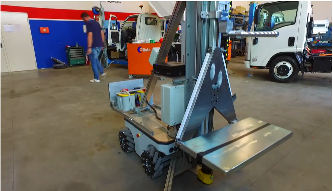
Figure 3: The steel plate mounted on the lower forks of the robot
