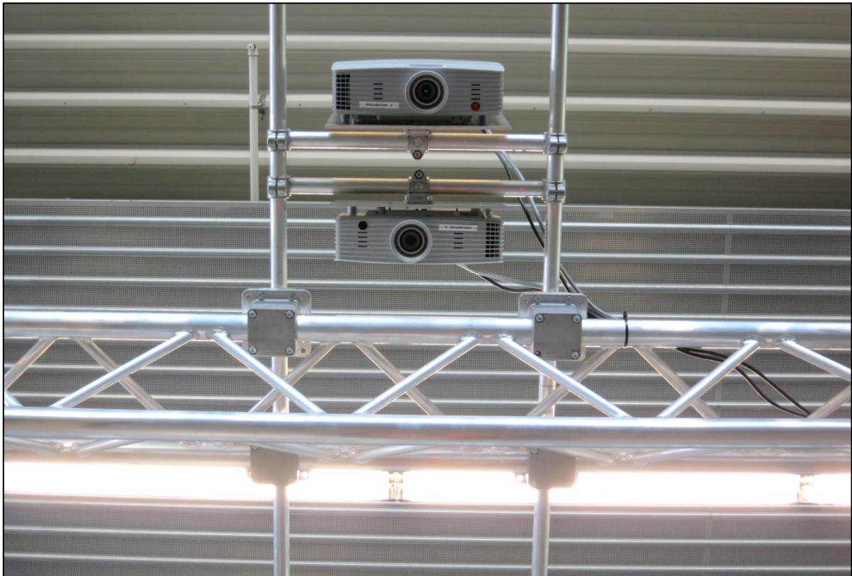
Figure 9: Projectors are mounted by an adapter plate and round pipes to the system carrier. The two projectors illuminate an area of 4.0 by 3.0 meters.
