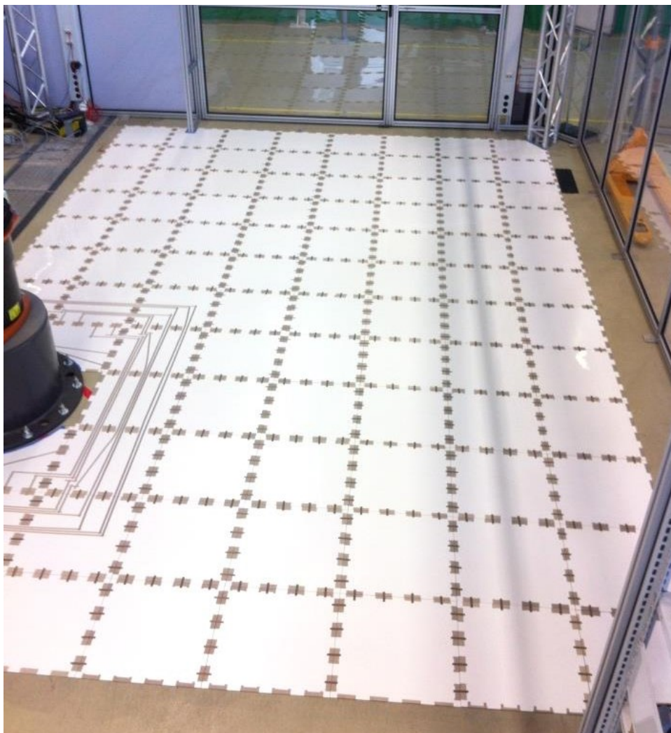
Figure 3: Finished buildup and wiring of sensor system that consists of single quadratic tiles and conductor band.
