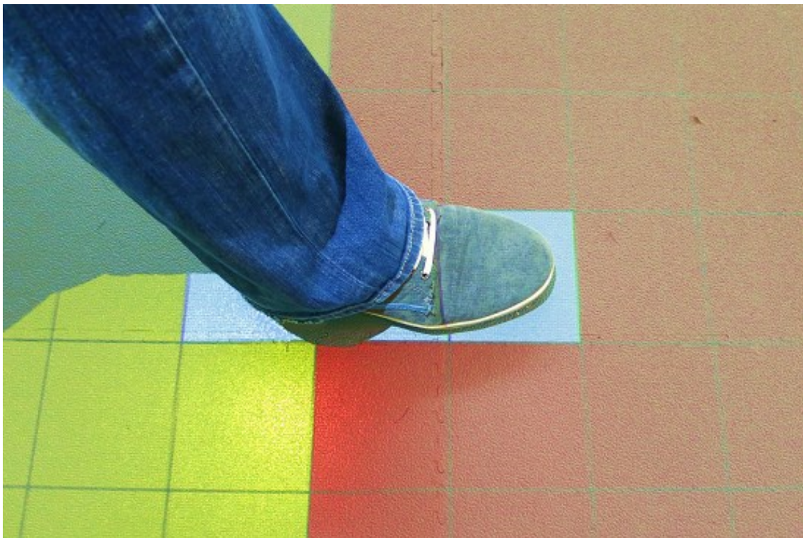
Figure 16: Triggered sensor cells are illuminated by the projection system. Warn area and critical are visualized.
