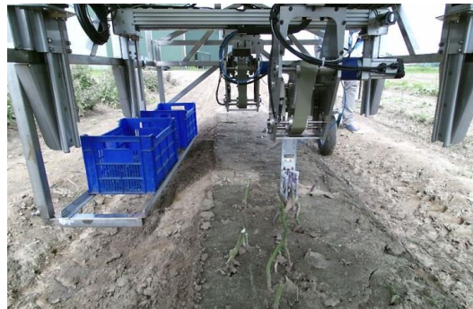
Fig. 1. The robotic harvester driving over an asparagus dam (a). The asparagus process as seen by the on-board camera. The storage box on the side of the machine (b).
