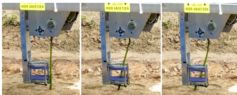
Fig. 2: Illustration of a part of the harvesting process, asparagus stalk approaching and grabbing by one of the harvesting tools
