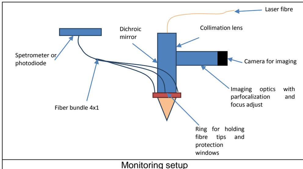
Hence, the experimental setup described here should allow us to measure most of the relevant characteristics of the laser process and thereby using the data for extracting information that can be used to implement a strategy for the control of the process.
