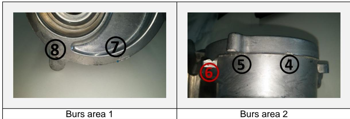
On the CAD, the areas of the part where burrs may appear are defined. The deburring trajectory of the robot is defined using the CAD.
