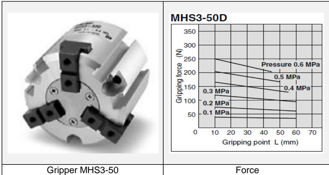
Parts required for manipulation on Debur project have a circular ring. For this reason the gripper has three fingers that may be manufactured depending on the part geometry to be grasped. The design of the gripper fingers has been done and manufactured.
