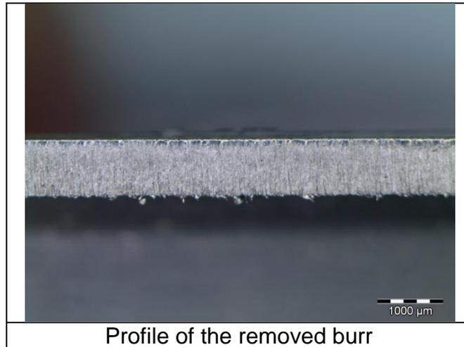
In the image of the removed burr cross section it can be seen a ribbed profile and small burrs, however finishing quality is quite good, as it is shown in the topography and cutting profile, obtained by a confocal microscope, of the following figure. The roughness achieved, measured in Ra, ranges between 2.5 μm and 3.0 μm.
