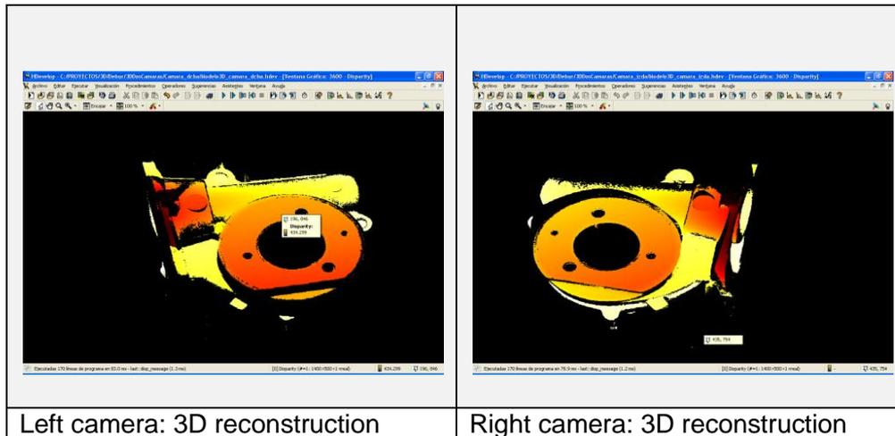
These two independent models have to be integrated into one to reduce the occlusions generated at each model. For the analysis of burrs, in the 3D workstation, the three principal steps were:
