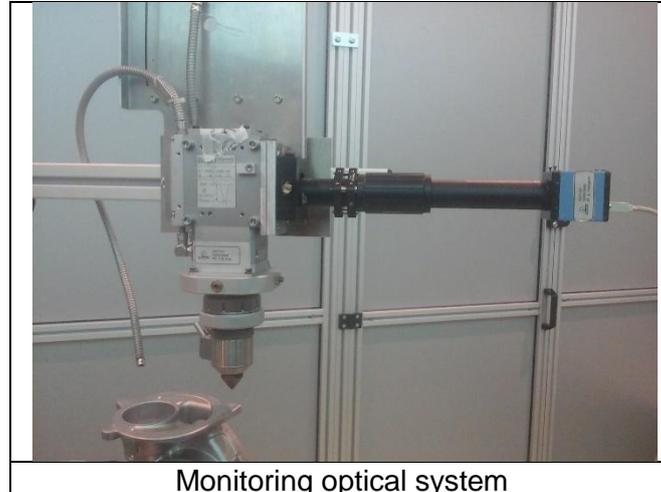
A deflection mirror has not been contemplated at first instance. So the number of optical elements is maintained at minimum and no additional restriction in the spectral range due to the use of a reflection coating for the mirror is introduced.
