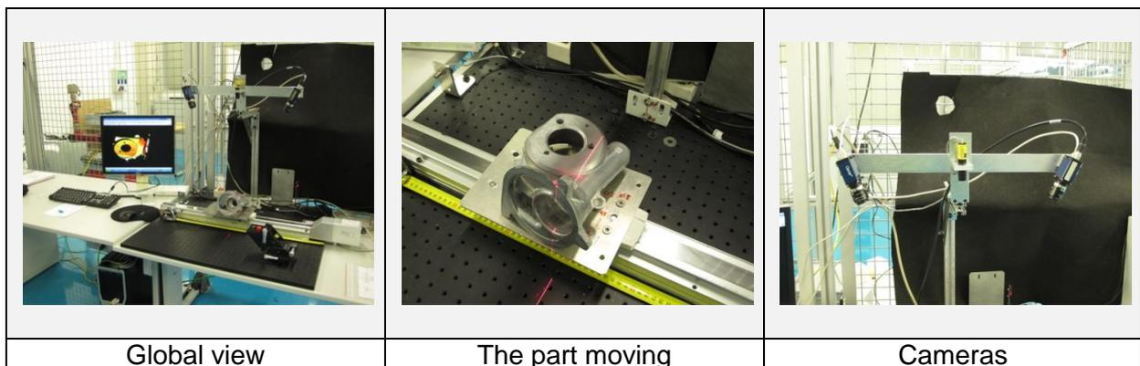
These images illustrate the constructed prototype. The left image is a global view showing the different elements: the linear axis, cameras, sheet of light and working station for development. The other two pictures shows a detail of the cameras and sheet of light and the moment where the part is being acquired by the vision system for posterior analysis.
