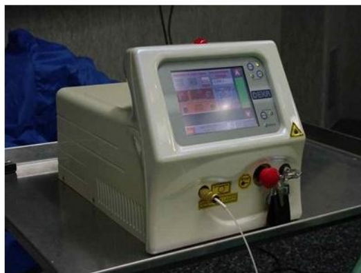
Fig. 11 - The diode laser currently in use for laser welding of the cornea (left), the fiber tip mounted in a handpiece (right).
