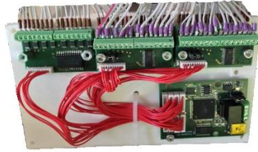
**Figure 4: Controller board for managing the sensor cells.**
