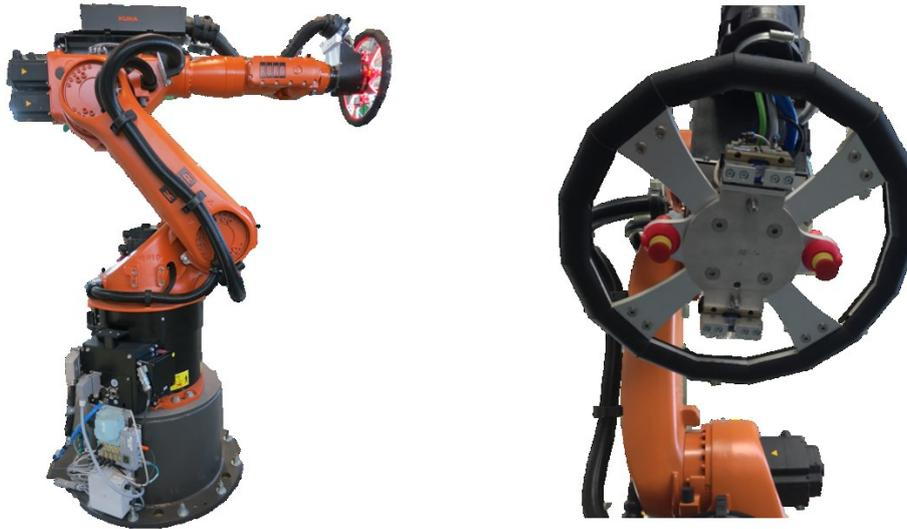
**Figure 3: KUKA KR60 L45 with additional operator device and gripper.**
