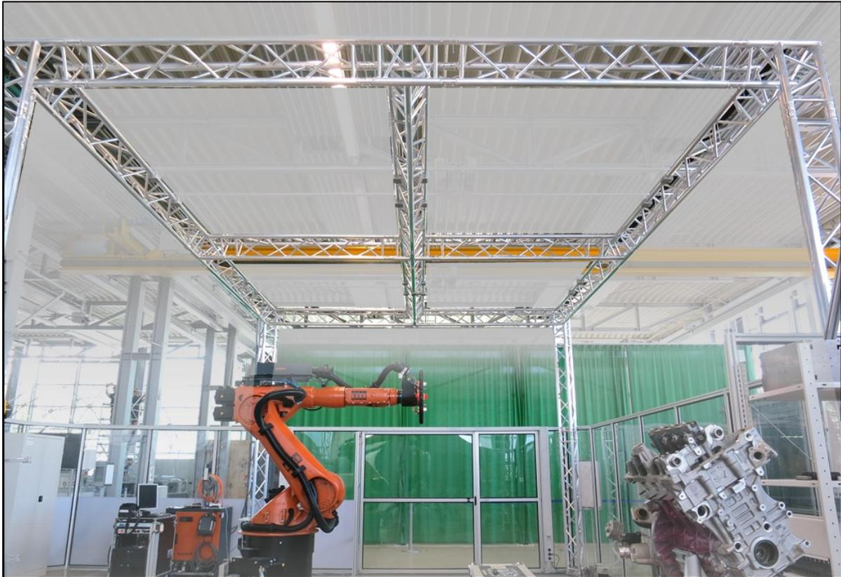
**Figure 2: System carrier for mounting the projectors.**
