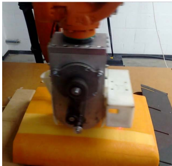
Figure 5: The robot motion on the cheese block while removing the coating.
