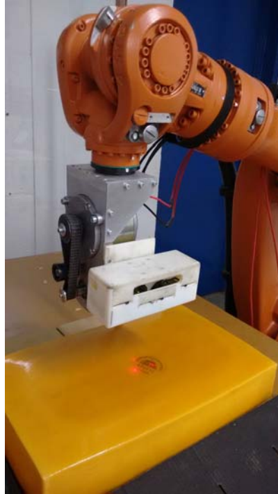
Figure 1: Experimental setup using KUKA KR16.
