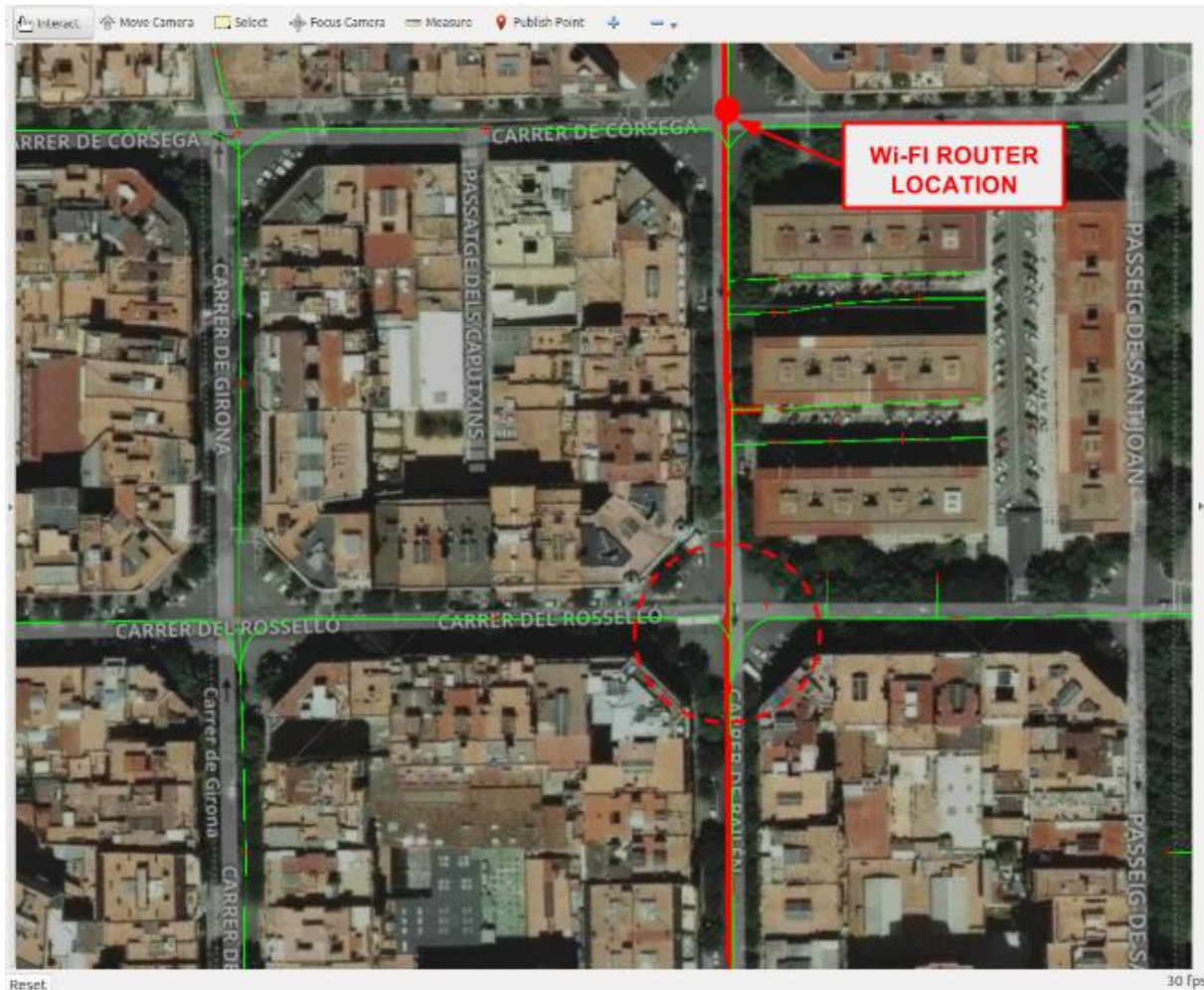
Figure 40: Wi-Fi propagation (in red) in Barcelona sewer tunnels (in green)
