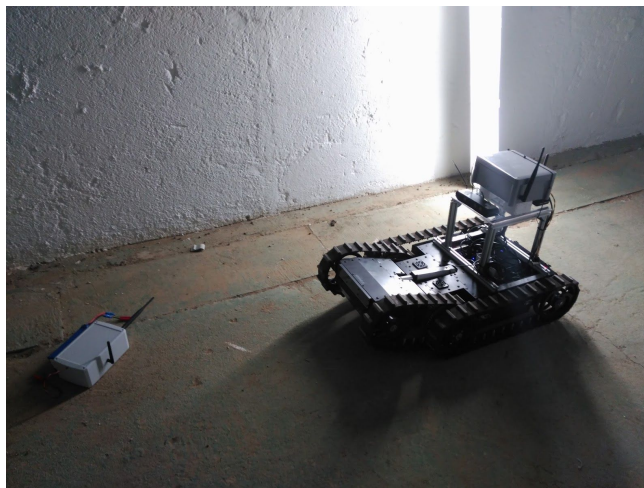
Figure 11. Communication experiments: the robot and one of the repeaters.
