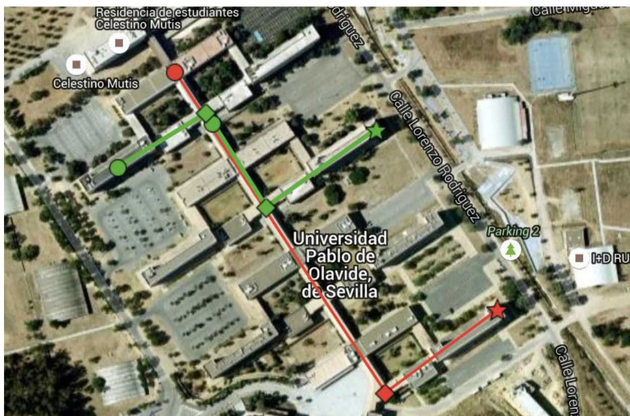
Figure 12. Communication experiments. Red: experiment with one repeater; the first leg is 330 m long, while the second is 120 m. Green: experiment with two repeaters; each leg is approximately 100 m long.
