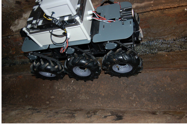
Figure 4. SIAR robot navigating in Valencia Street sewer
