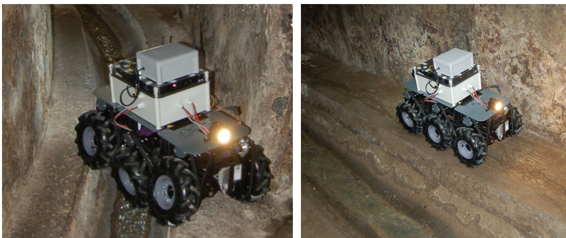
Figure 9. SIAR first prototype sewer experiments.
