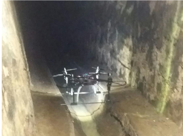
Figure 2: Validation of the adapted landing gear for specific sewer sections
