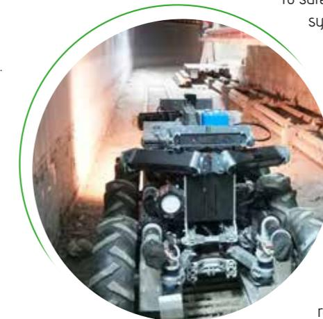
To safely navigate through the sewage system while following an inspection plan, the robot can be localized at any time. Thanks to the onboard sensors and given prior geometric information of the sewer's structure **SIAR** is capable to self-localize in real-time with an absolute error below 1m.
