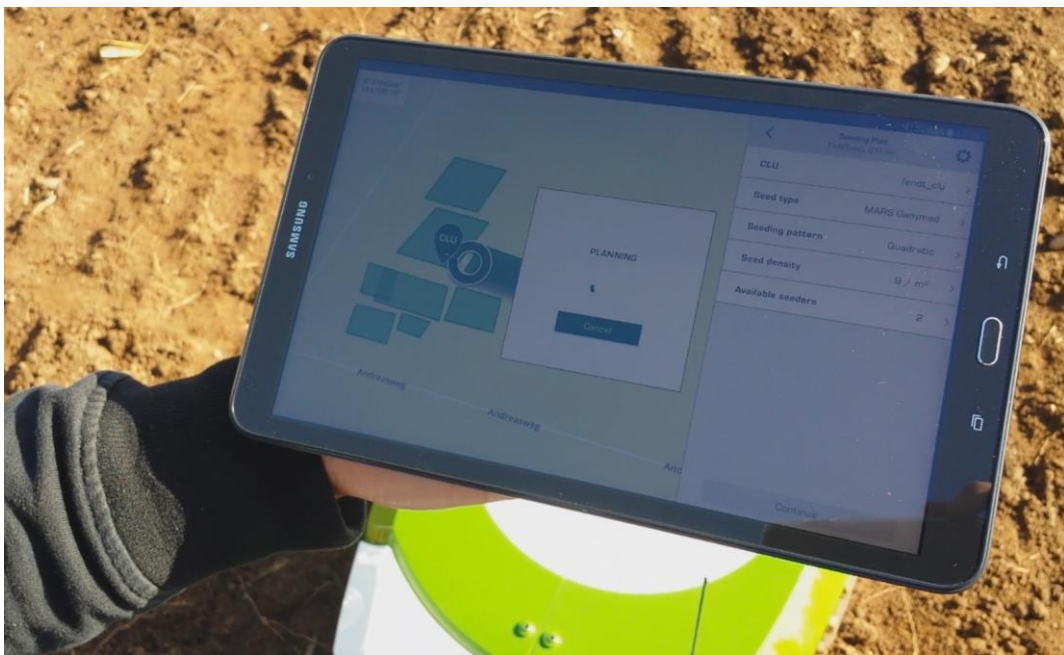
Figure 26: Planning of seeding task (field selection, parameter adjustment).
