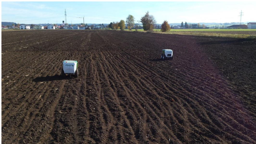
Figure 28: Robots executing the seeding task.
