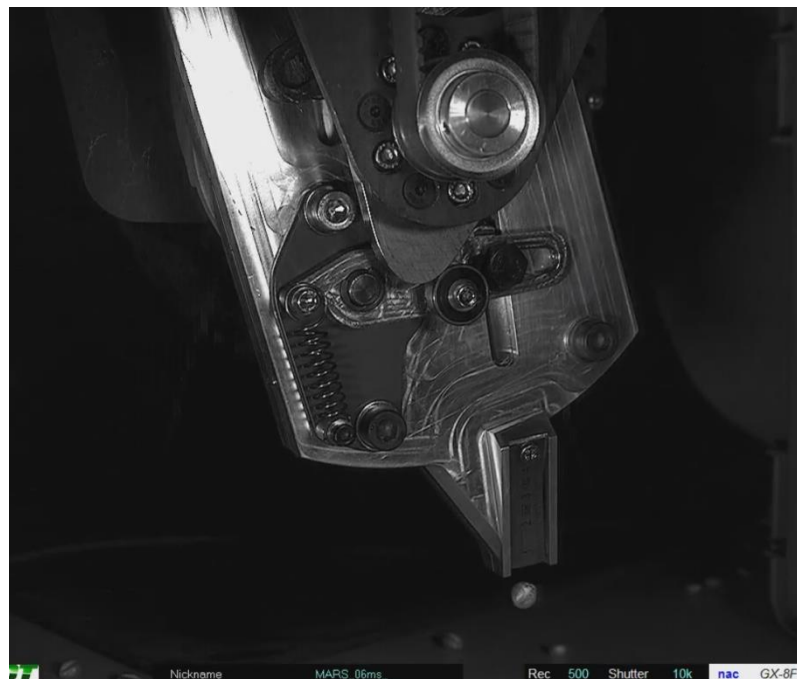
Figure 21: Still frame taken from high speed recording of seeding unit during laboratory test.
